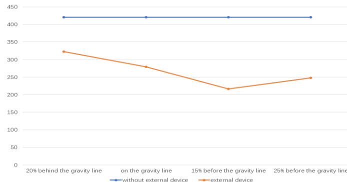
Figure 22. Maximum deformation for cases with external device at difference positions.
