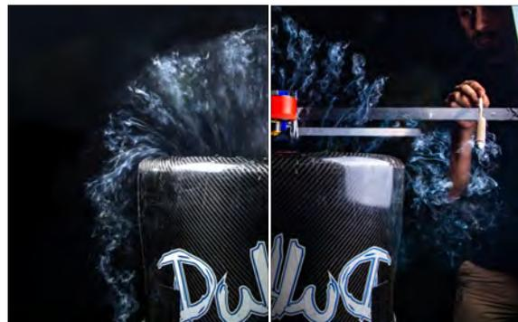
Figure 12: Smoke visualisation test for the reference position
