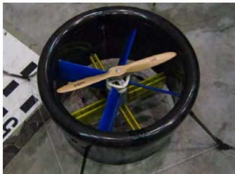
Figure 1: The ducted fan MAV of ULB, Dulbema.
