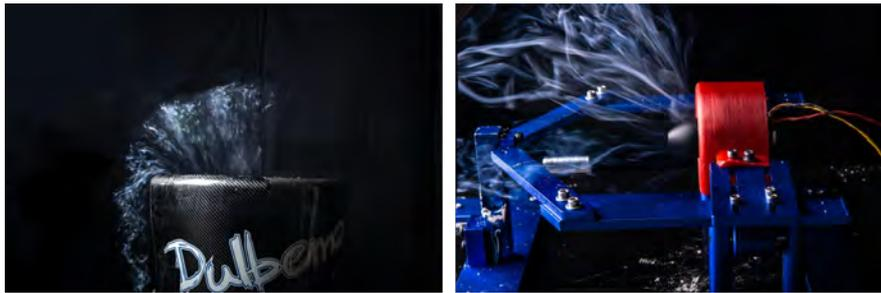
Figure 11: Smoke visualisation results obtained for Dulbema (left) and EDF (right)
