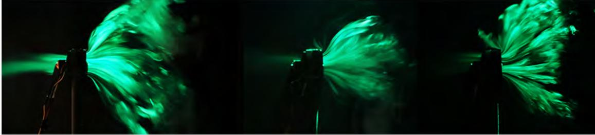
Figure 16: Visualization of the flow for  $200 g_F$  from left to right: CCW manufacturer, CW printed, CCW printed
