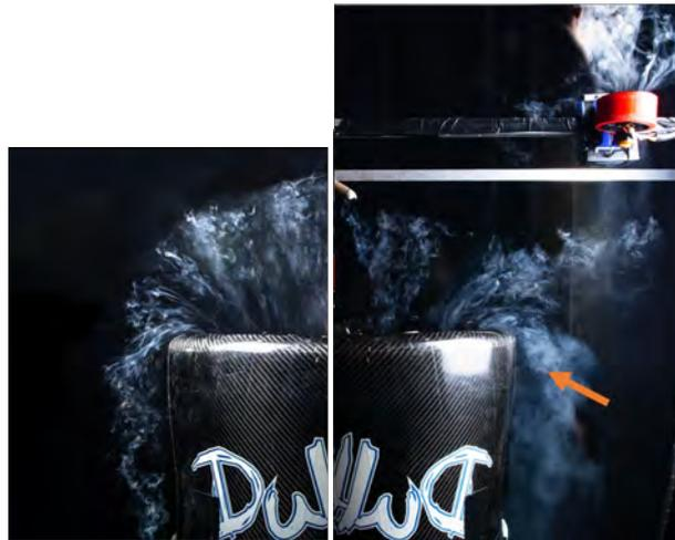
Figure 13: Smoke visualisation test for the C position
