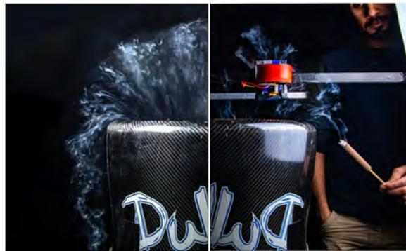
Figure 14: Smoke visualisation test for the P position
