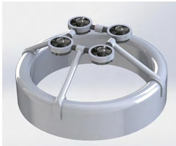
Figure 5: SaFly's control stage for pitch and roll
