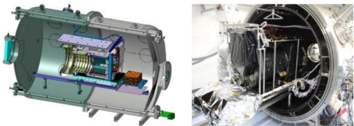
Figure 5: Thermal vacuum chamber set up at UBE (left) , flight model installation (right)
