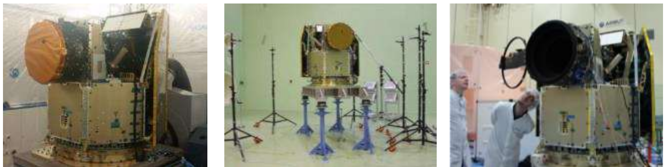
Figure 6: Spacecraft SQM model during sine vibration test (left) SQM during acoustic test (center) opening of the cover following mechanical test campaign (right)
