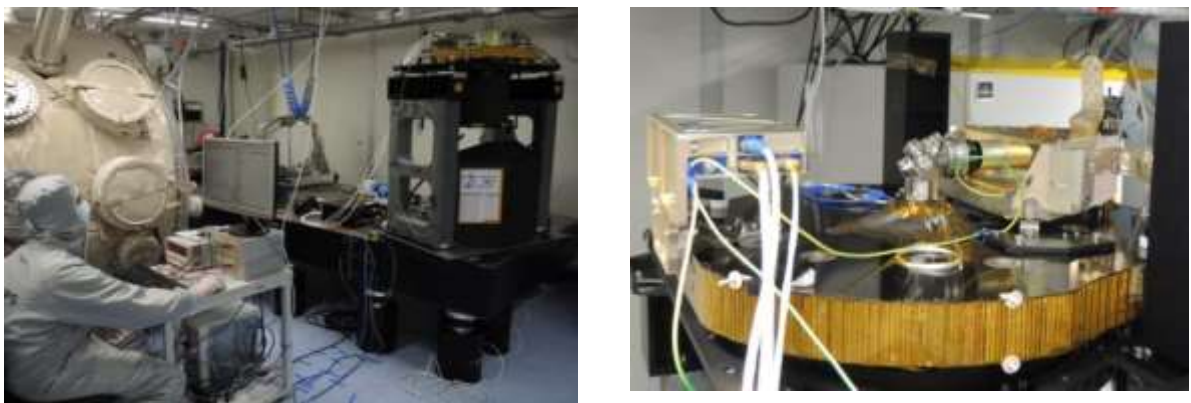
Figure 7: Cheops telescope with FPM EM/EQM/FM during alignment (left) Focal plane module EM/EQM mounted and aligned on optical bench (right)
