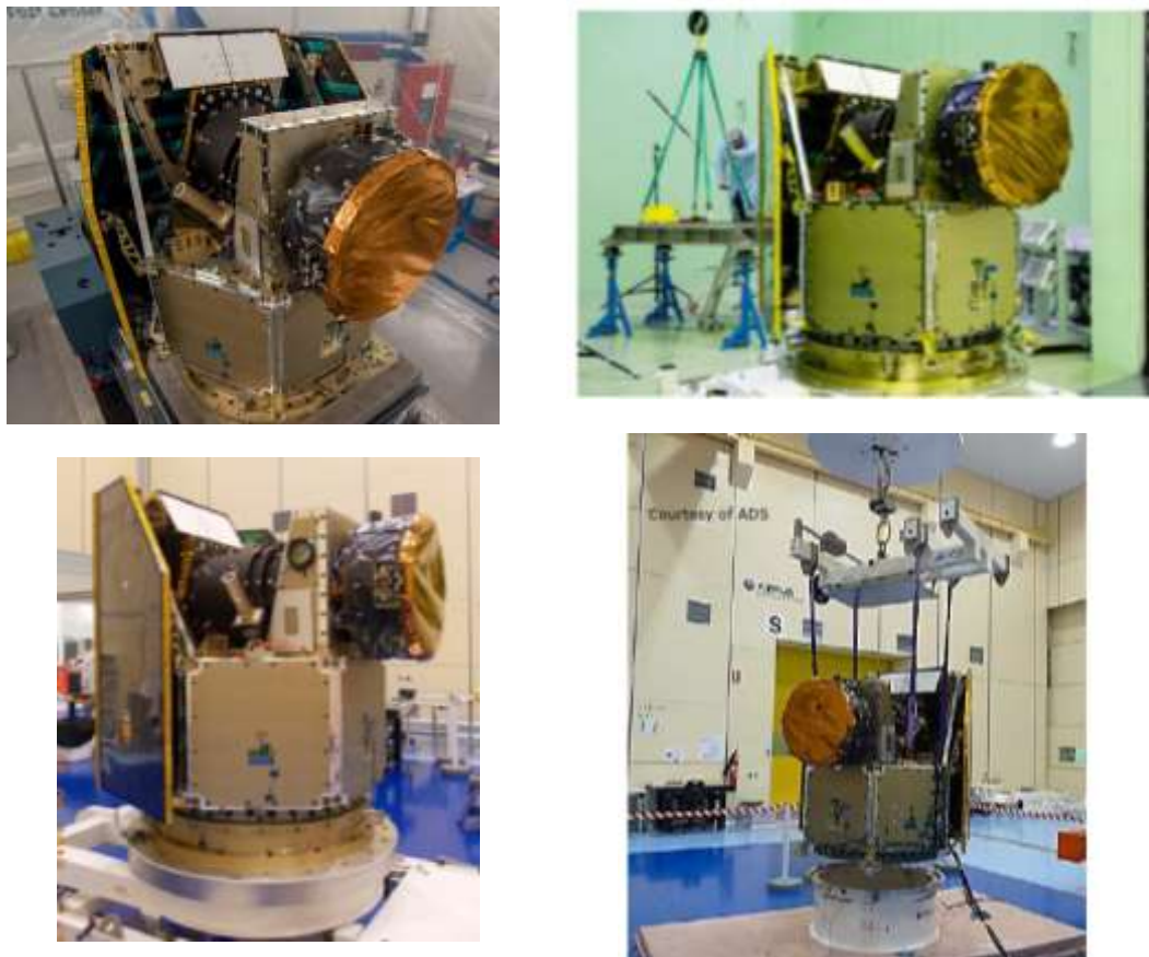
Figure 9: Top left Satellite Structural Model (STM) undergoing vibration tests (courtesy of RSSZ-CH), top right during acoustic test at ESTEC (courtesy of ETS), bottom left during mass measurement and bottom right during shock test (courtesy of ADS Spain).
