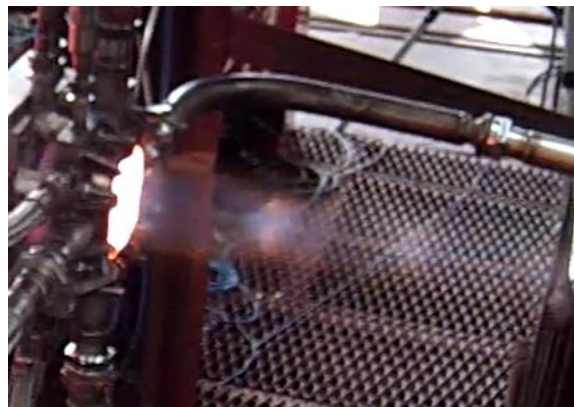
Figure 5: Photo of thermal radiation shock waves in high temperature test jet.
