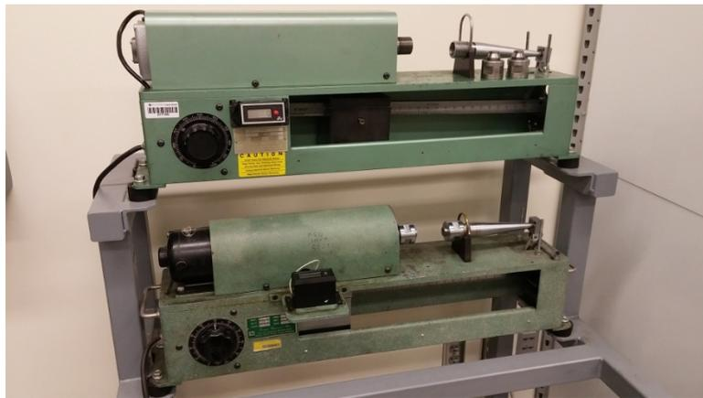
Figure 2: Model RFB200 fatigue tester by Fatigue Dynamics. (Image by authors.)
