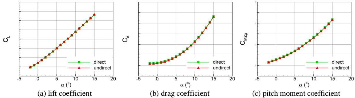
Fig. 9: 20 degrees rudder symmetric deflection
