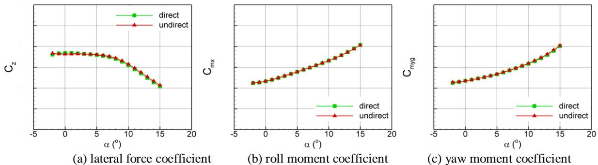
Fig. 10: 20 degrees rudder asymmetric deflection
