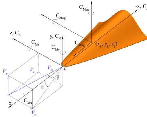
Fig. 1: Definition of the body axes system.
