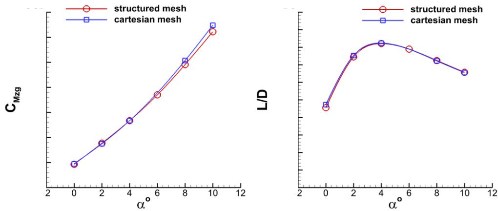
Fig. 2: Aerodynamic coefficients calculation results using different types of mesh
