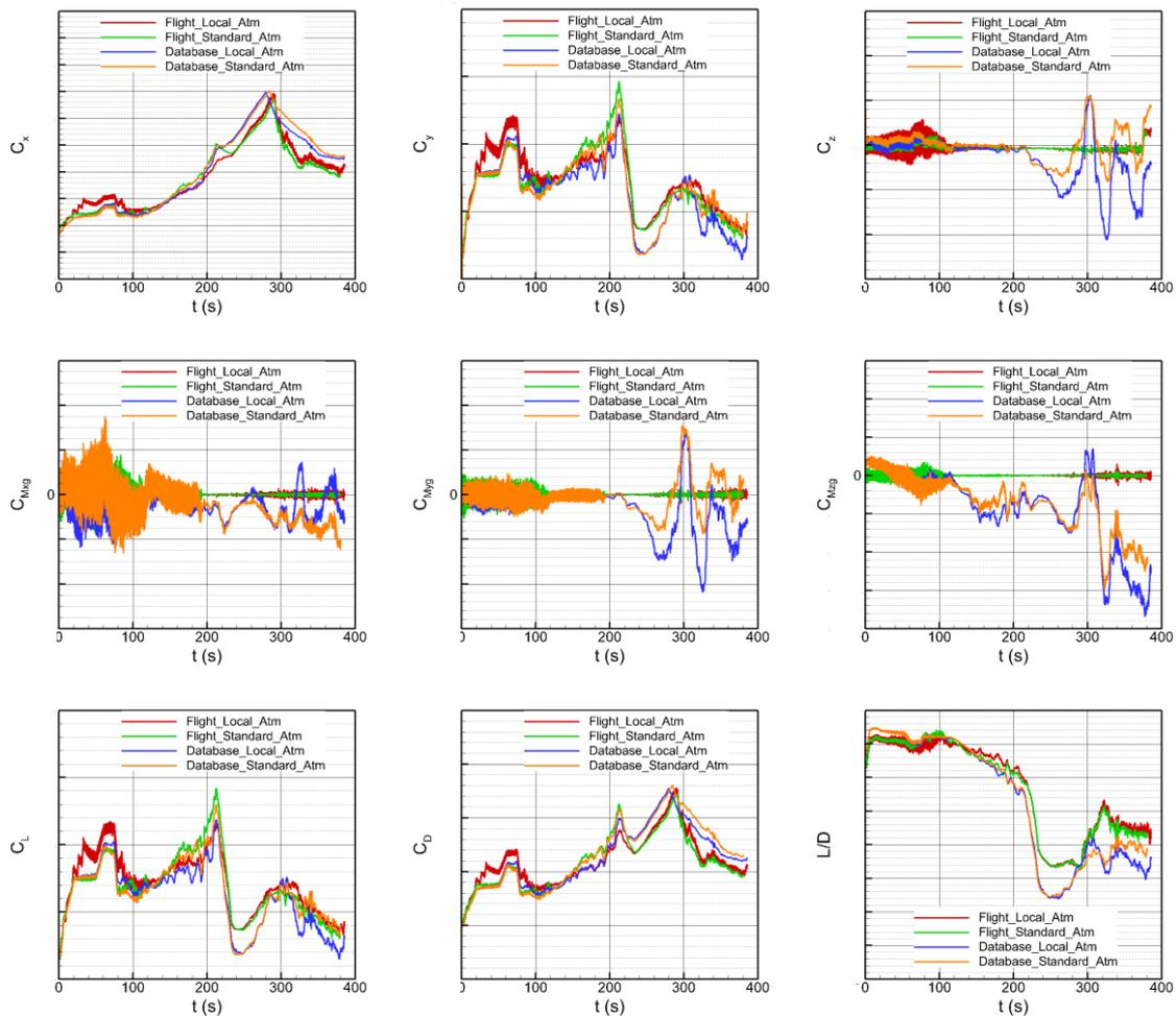
Fig. 12: Comparison between flight data and database prediction
