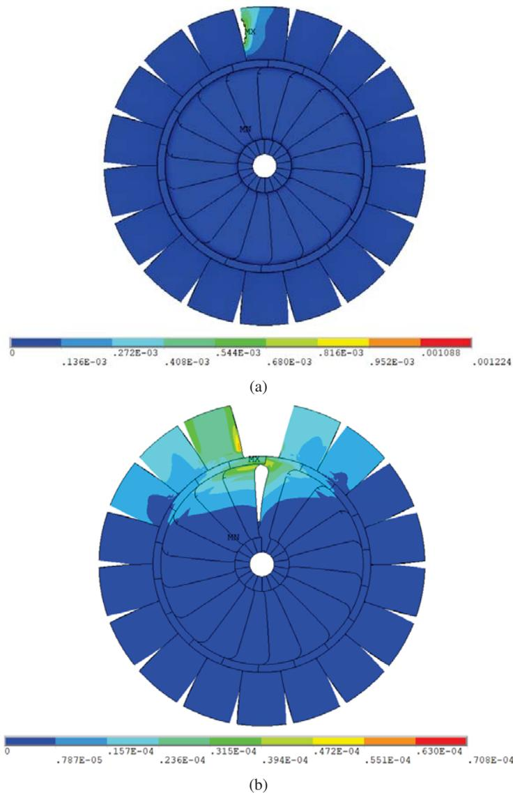
Figure 8: Visualization of the error metric between the prestressed *pristine* and *mistuned* stiffness  $\mathbf{K}_{var}$
