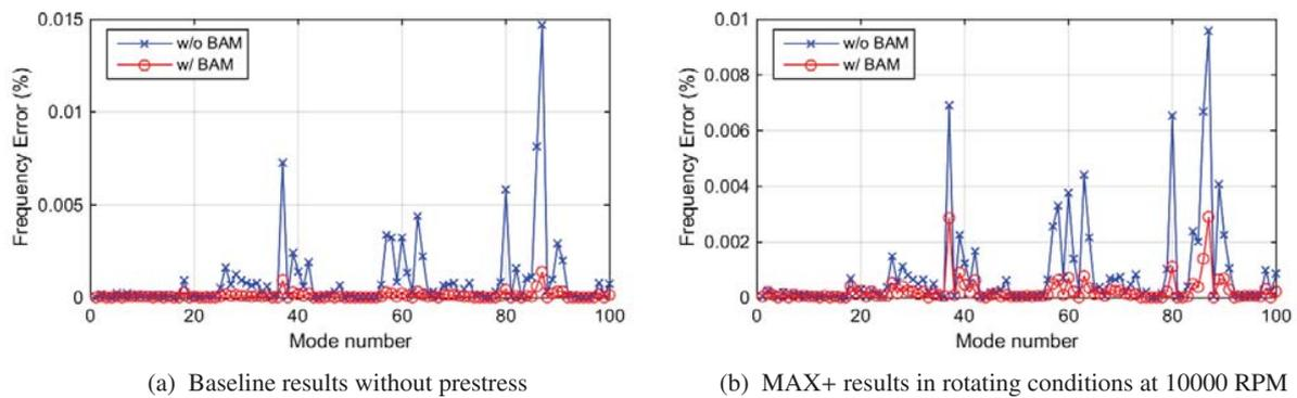
Figure 9: Validation results obtained in different prestress conditions for the IBR of Figure 3
