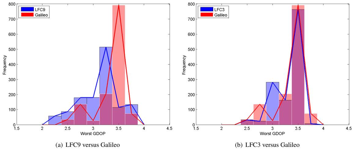
Figure 7: Worst GDOP comparison of designed LFC and Galileo
