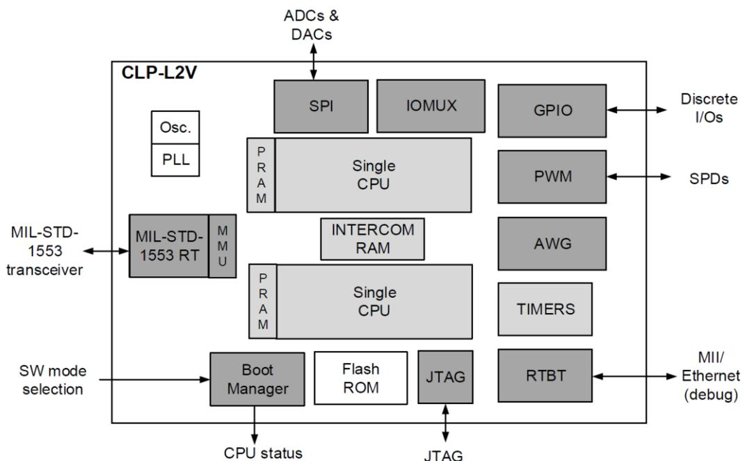
Figure 4: Vega-C specific CLP processor architecture
