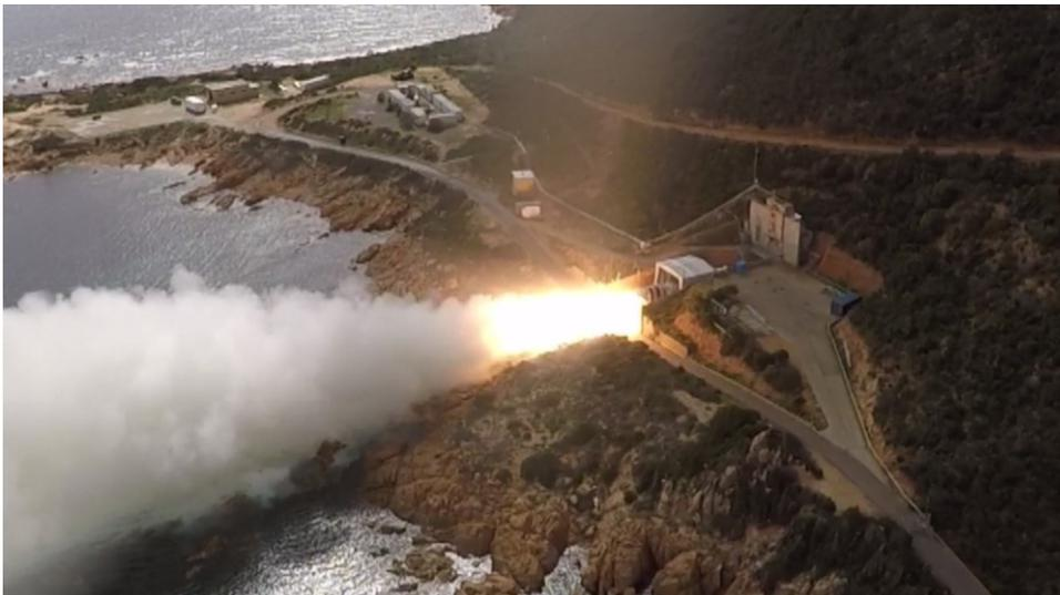
Figure 5: Aerial view of the Z40 development model static firing test in Sardinia, Italy
