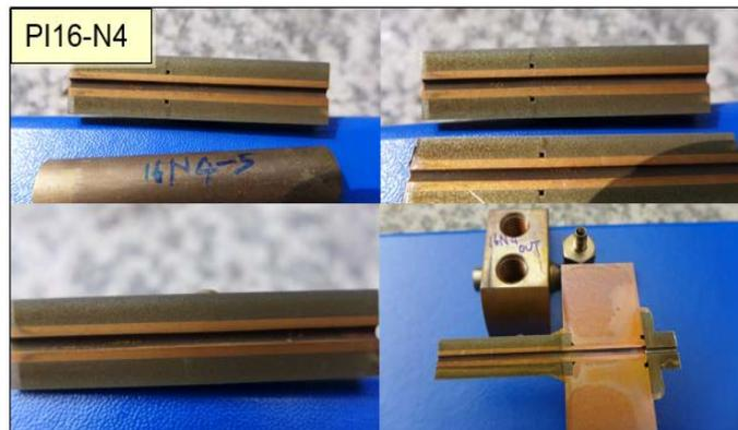
Figure 13: Cut-off photograph of the specimen after 6<sup>th</sup> coking test
