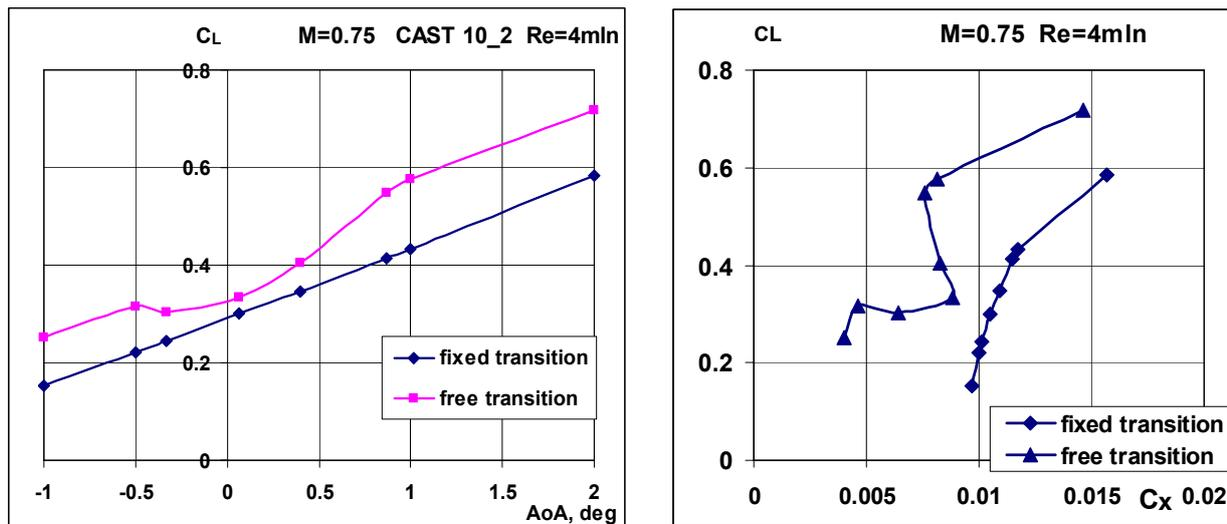
Figure 5: Computational results of the BLWF solver. Dependence of lift coefficient on angle of attack (a) and drag polar (b) at  $M=0.75$  for fixed and free transition.
