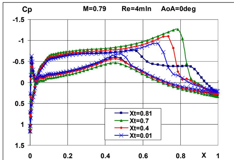
Figure 7: Influence of transition point  $x_t$  on the pressure distribution of the wing CAST.  $M=0.79$ ,  $Re=4\text{mln}$ , angle of attack  $AoA=0$ .
