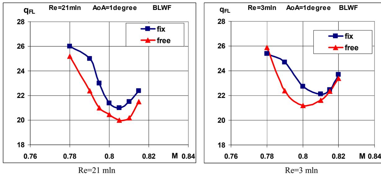
Figure 17: Effects of viscosity and flow transition on flutter dynamic pressure.
