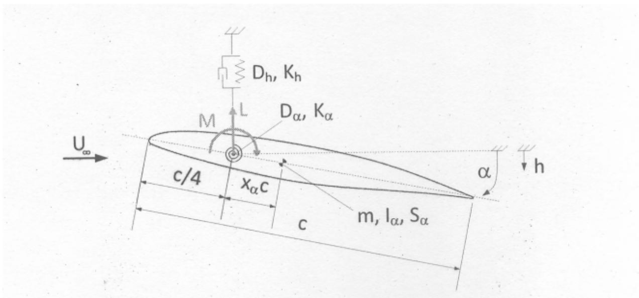
Figure 2: Computational CAST model for flutter analysis from [11].
