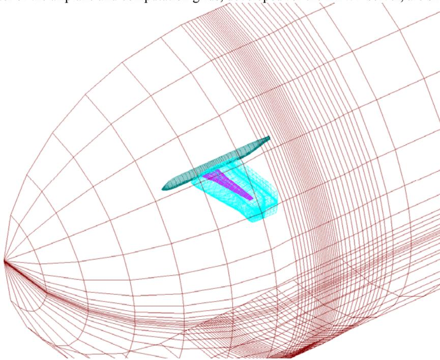
Figure14: Aerodynamic model and computation grids for the BLWF solver
