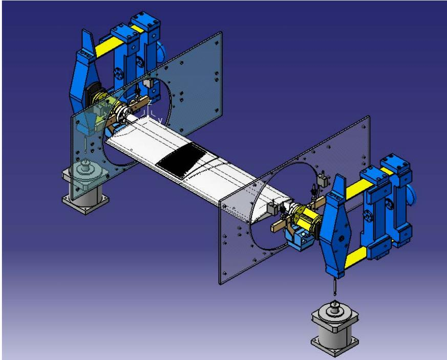
Figure 1: Two-dimensional CAST model in transonic WT TWG [11].
