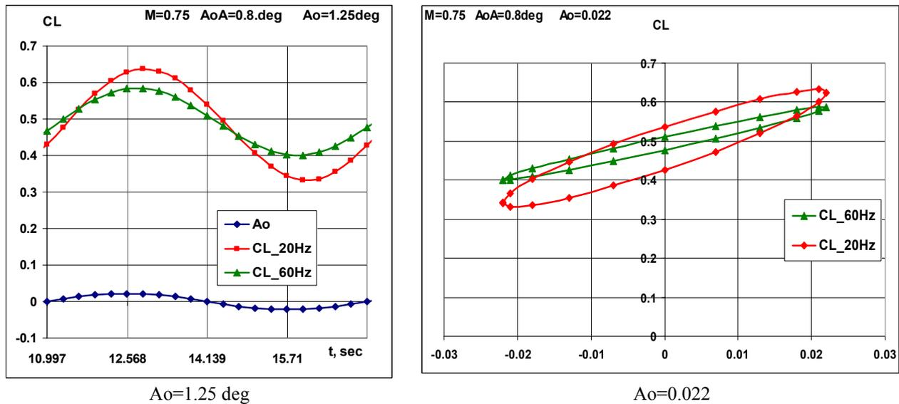
Figure 12: Change in the lift coefficient over one period for pitch motion at  $M=0.75$ ,  $AoA=0.8$  degree, LCO amplitude  $Ao=1.25$  degree.
