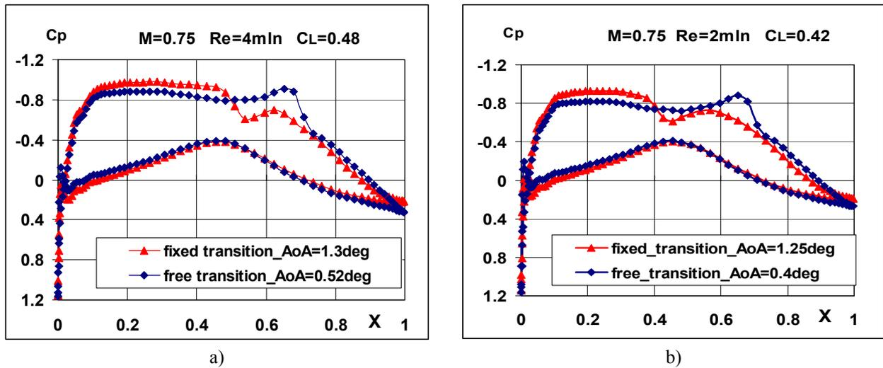
Figure 6: Pressure distribution at Mach number  $M=0.75$  for fixed and free transition for two different flow regime: a)  $Re=4\text{mln}$ ,  $CL=0.48$ , b)  $Re=2\text{mln}$ ,  $CL=0.42$ .
