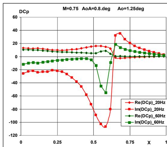
Figure 13: Real and imaginary parts of the lift coefficient response to pitch motion.
