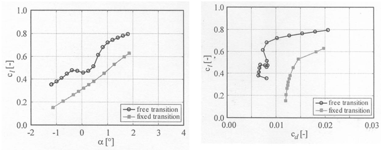
Figure 4: Experimental results from [9]. Lift curve (a) and drag polar (b) for  $M=0.75$  at fixed and free transition.
