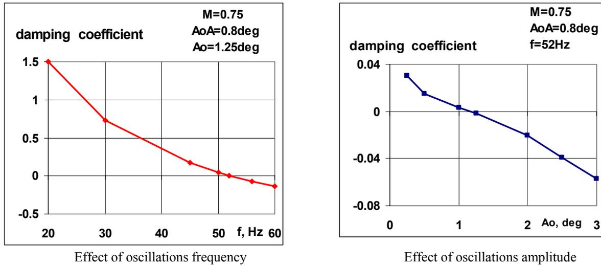
Figure 11: CAST model pitch motions. Dependence of damping coefficient on frequency (a) and amplitude (b) at  $M=0.75$ ,  $AoA=0.8$  degree.
