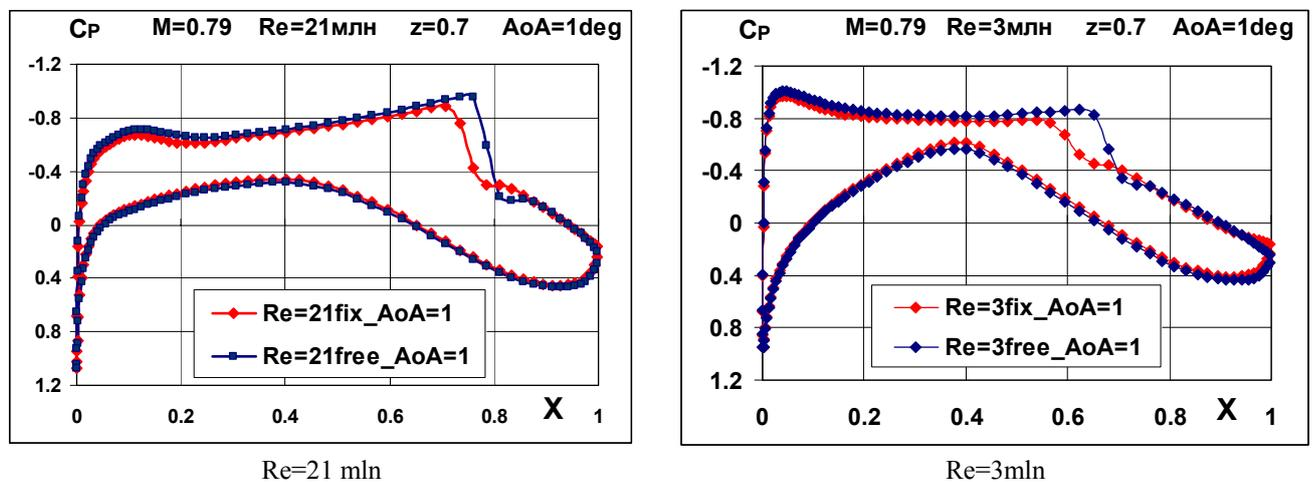
Figure 15: Comparison of pressure distributions for two flow regimes:  $Re=3$ mln and  $Re=23$ mln, turbulent and transitional flow at  $M=0.79$  for wing section  $z=0.7$ .
