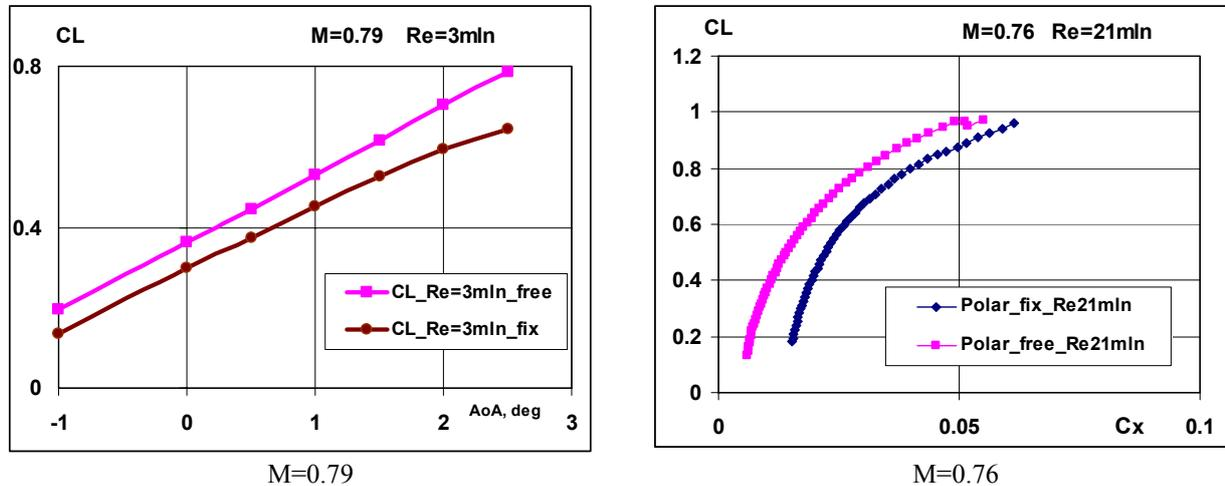
Figure 16: Lift coefficient and drag polar for turbulent and transitional flows.
