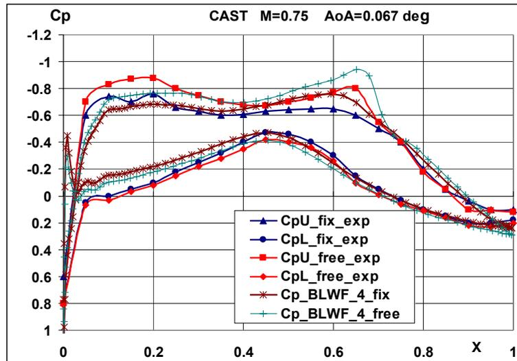
Figure 8: Pressure distribution on the CAST 10-2 airfoil for free and fixed transition. Comparison of analysis and experiment [6, 9-11].
