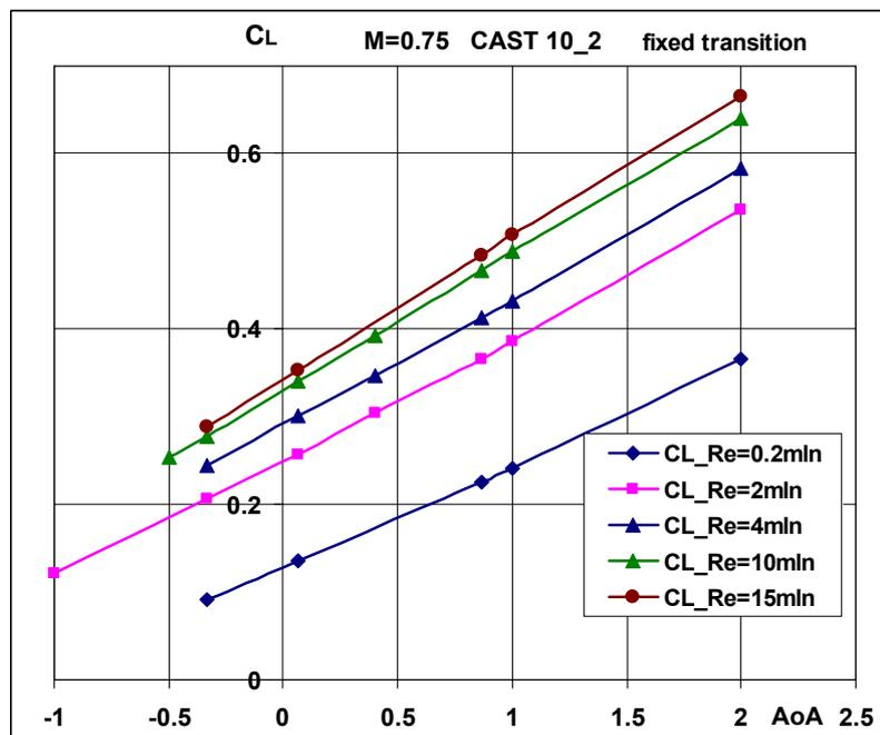
Figure 3: Results of the BLWF program computation. CAST model. Fixed point of transition. Effect of Reynolds number on lift coefficient at  $M = 0.75$ .
