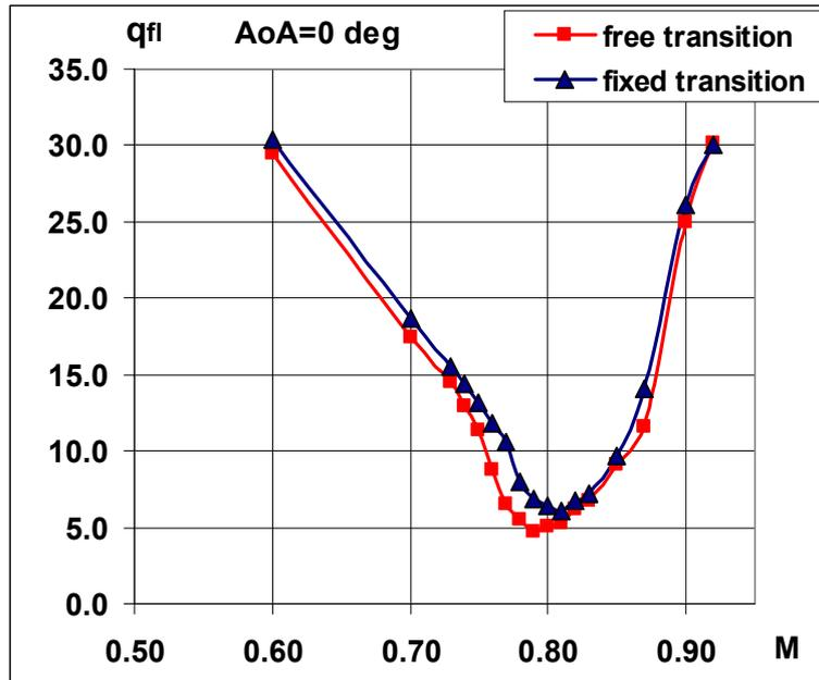
Figure 10: Dependence of flutter dynamic pressure on Mach numbers for two flow regimes.
