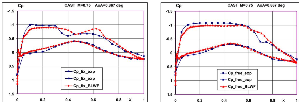
Figure 9: Comparison of pressure distribution on the CAST 10-2 airfoil for free and fixed transition. Results of analysis and experiment [6, 9-11].
