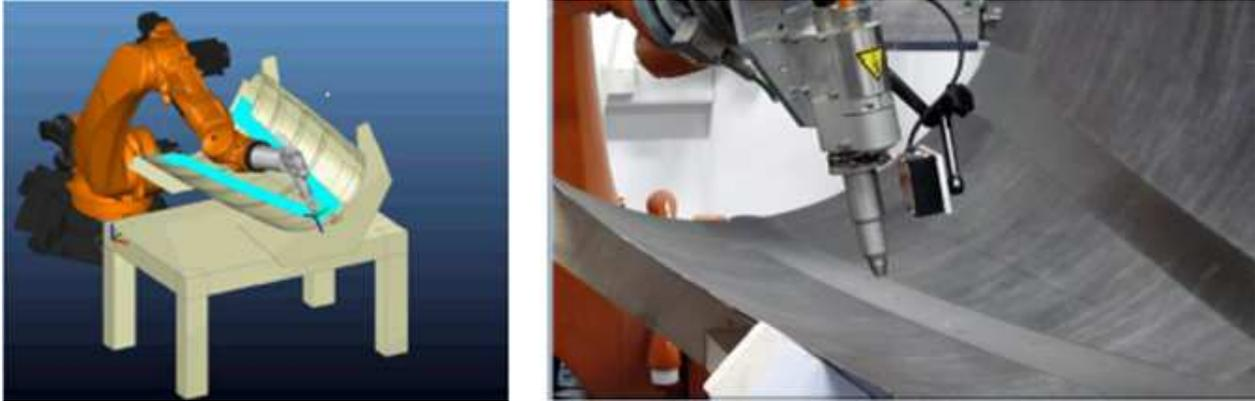
Figure 14: Automatic plasma treatment prior to bonding
