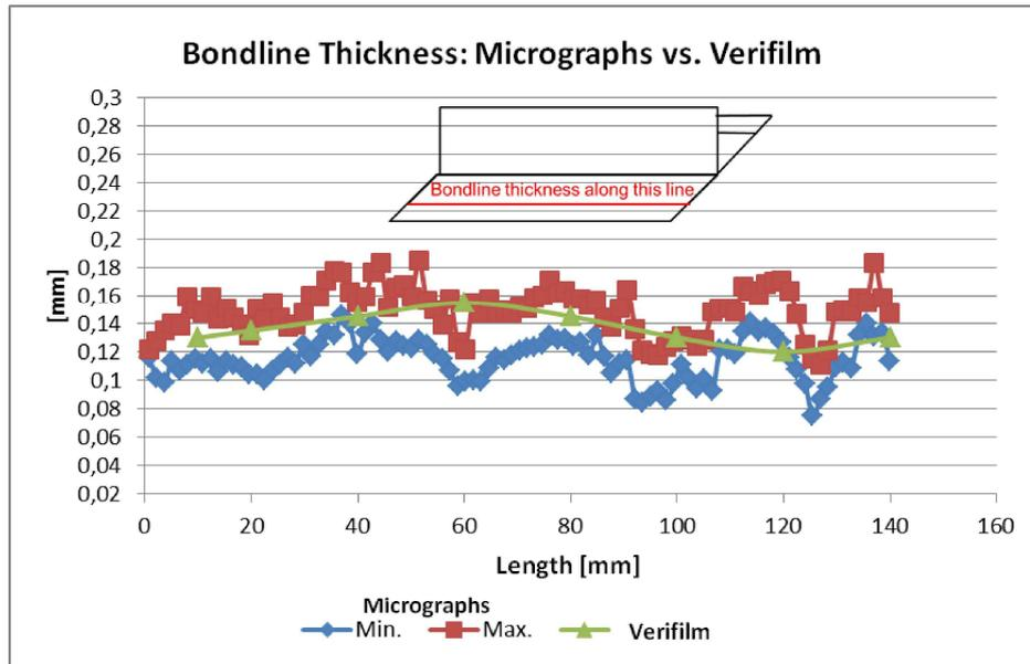
Figure 12: Bondline thickness: Micrographs vs. Verifilm
