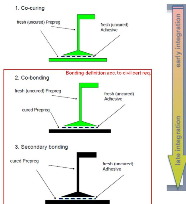
Figure 2: Composite manufacturing and assembly joining technologies
