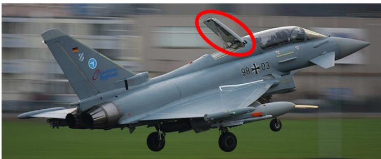
Figure 6: Eurofighter Typhoon (EFA) with deployed airbrake
