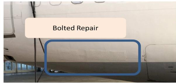
Figure 4: Bolted fuselage repair
