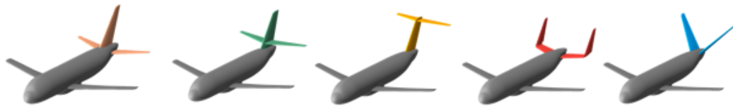
Figure 3 - Empennage concept down-selection
