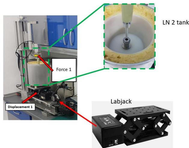
Figure 5: The LN2 test bench for component characterization
