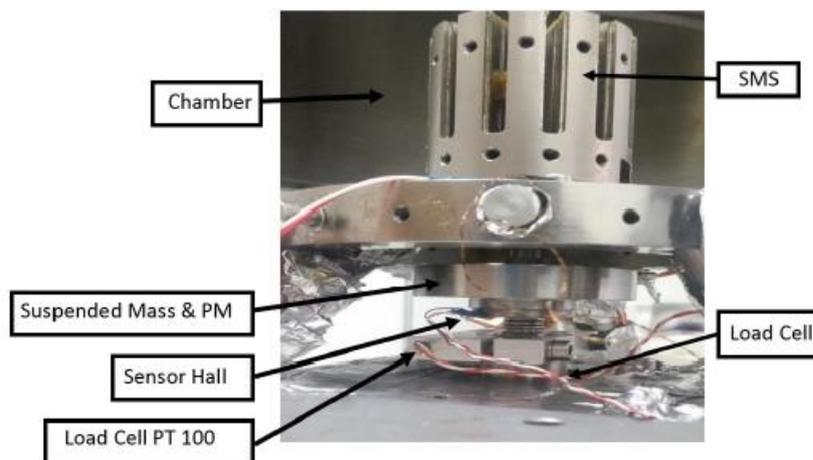
Figure 10:Free oscillation test-bench
