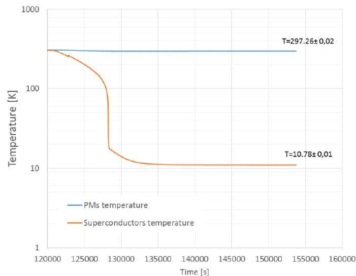
Figure 3: Thermal disconnect feature (null thermal conductivity)
