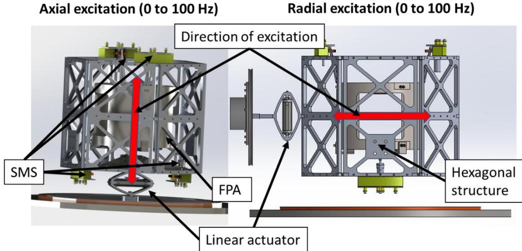
Figure 4: Axial and Radial test bench for FPA characterization
