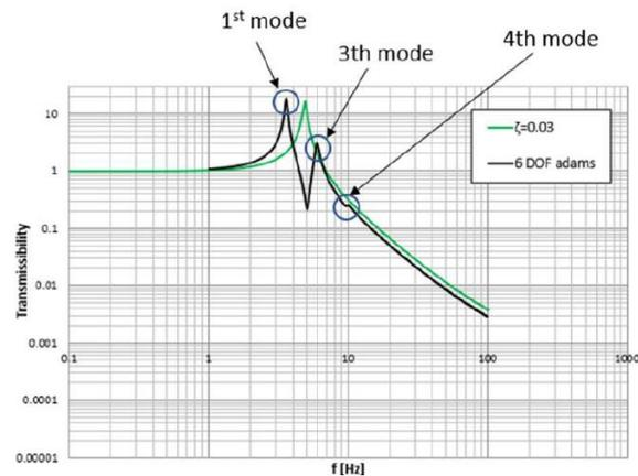
Figure 2: 12 kg FPA transmissivity from 0 to 100 Hz
