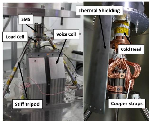
Figure 8: Axial characterization test bench
