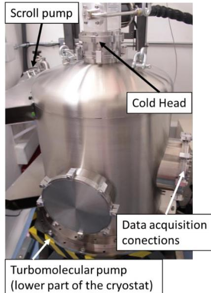
Figure 7: Vacuum chamber with 4K Cold Head
