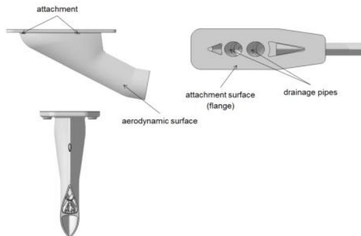
Figure 16: AM Drain mast. Final design
