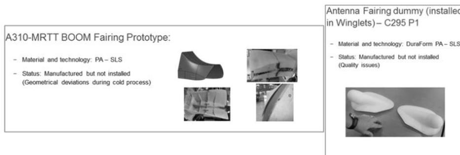
Figure 21: AM prototypes not suitable to install in aircraft
