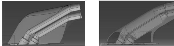
Figure 15: AM Drain mast. Preliminary designs
