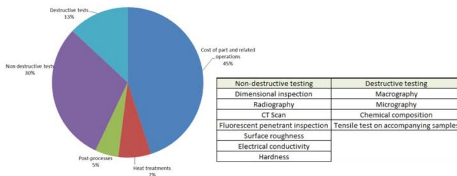
Figure 6: Cost break-down of the manufacturing of an aluminum part by SLM
