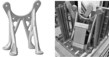
Figure 20: Fuel Pipe Bracket AM Design and Production Batch
