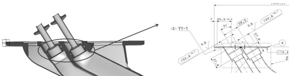
Figure 14: Drain mast. Angle of drainage piping
