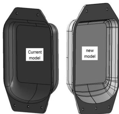
Figure 10: Current versus ALM design of the cover
