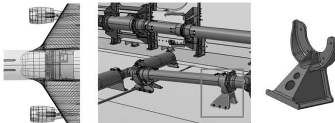
Figure 18: Fuel Pipe Bracket. Candidate selected for Scalmetalloy Topology Optimized Prototype
