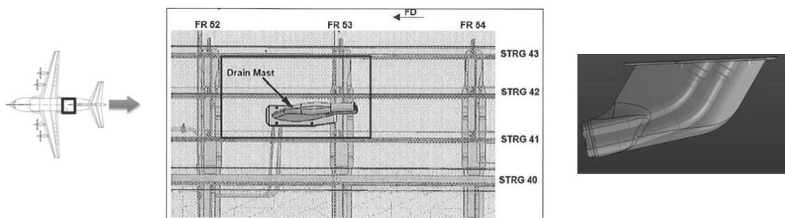
Figure 12: Drain mast location in the A400M
