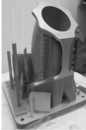
Figure 5: Opening in support structure to ease powder aspiration in AAR System of MRTT aircraft
