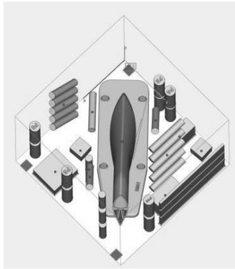
Figure 17: Drain mast. Batch Configuration
