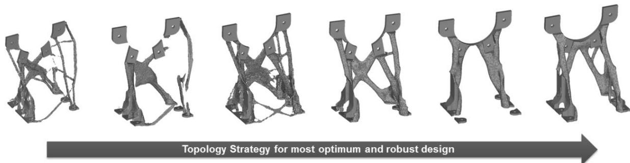
Figure 19: Fuel Pipe Bracket Topology Optimization Evolution
