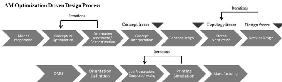
Figure 2: Optimization Driven Design Process for an AM Part
