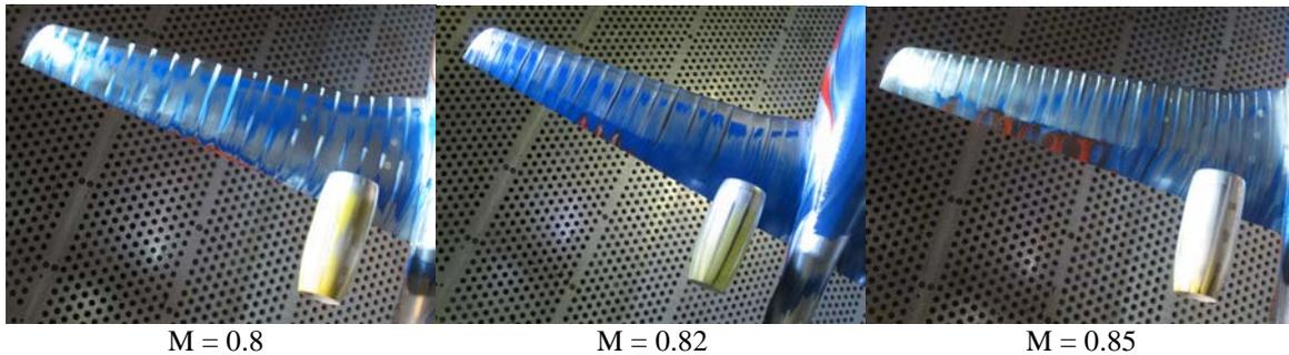
Figure 8: The flow visualization at different Mach numbers ( $\alpha = 1.5^\circ$ ) by colored oil film technique
