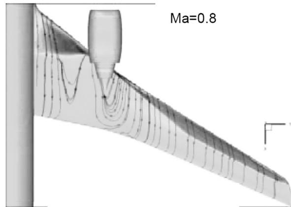
Figure 1: Shock-induced separation inboard of the pylon on the over-wing-nacelle configuration
