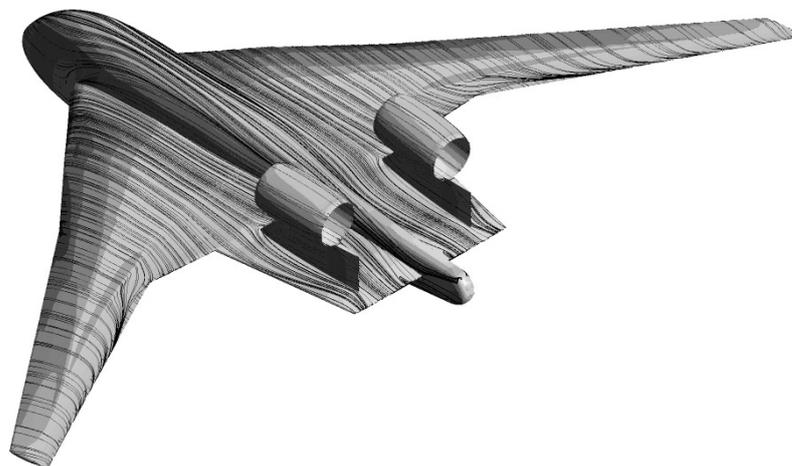
Figure 10: CFD flow field visualization over a novel FW configuration
