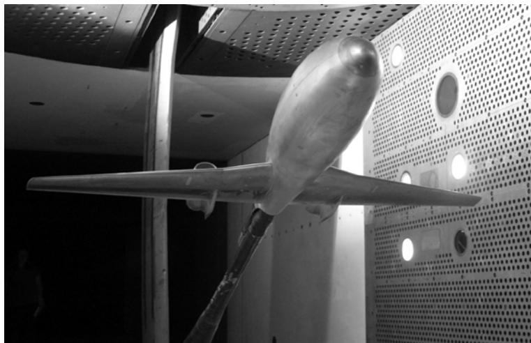
Figure 7: The business jet aerodynamic model with engine over-wing arrangement
