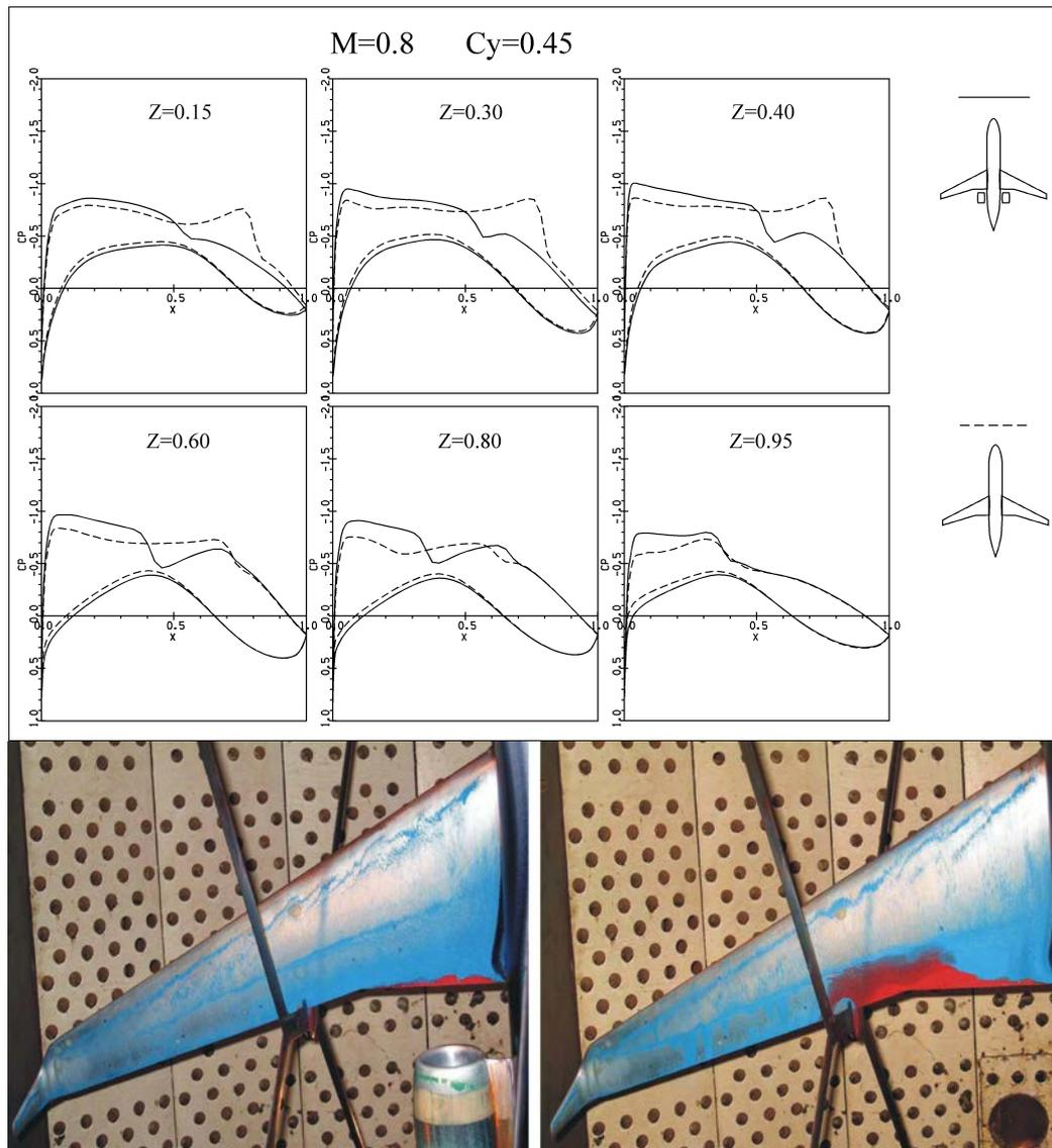
Figure 3: Suppression of the shock-induced flow separation by the nacelle installation (the T-106 wind tunnel experiment)
