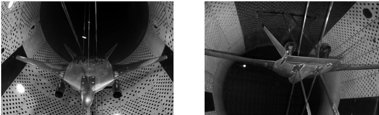
Figure 9: The FW aerodynamic model with forward under-wing and rear over-wing nacelles arrangements
