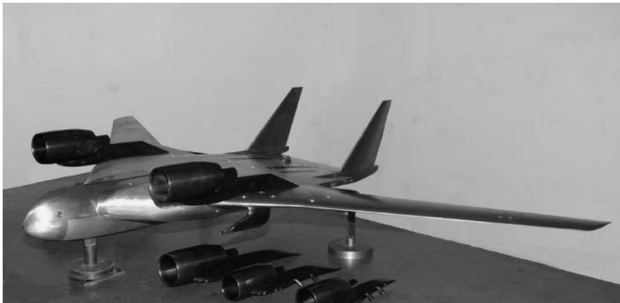
Figure 2: TsAGI “Flying Wing” aerodynamic model with the upper nacelles forward position
