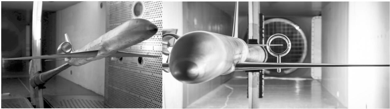
Figure 4: The aerodynamic models of low-sweep wing (LSW-2, LSW-3) regional aircraft with over-wing nacelles
