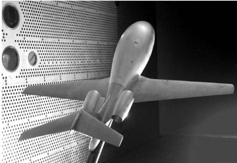
Figure 6: The “Tadpole” business jet aerodynamic model with straight wing ( $M_{\text{cruise}} = 0.8$ )
