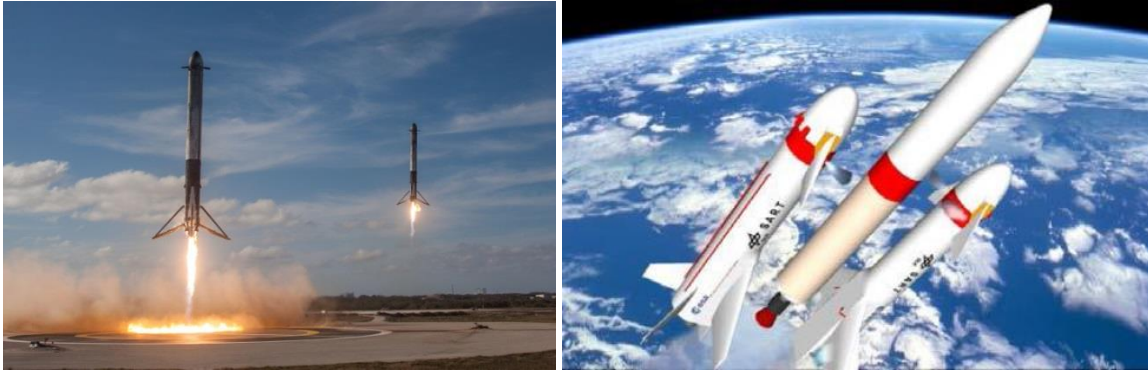
Figure 1: SpaceX Falcon Heavy side booster using the VTVL method (left; photo by SpaceX ; CC0 1.0) and the LFBB representing the VTHL method (right) [1]
