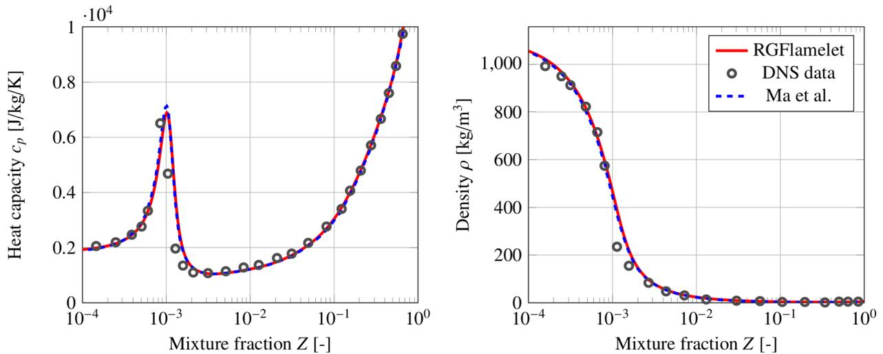
Figure 3: Validation of the real gas flamelet solver RGFlamelet using results from Ma et al.<sup>15</sup> and DNS data from Lacaze et al.<sup>14</sup> The plot shows the flame structure for a  $\text{H}_2/\text{O}_2$  counter flow diffusion flame with transcritical oxygen injection at 7 MPa.
