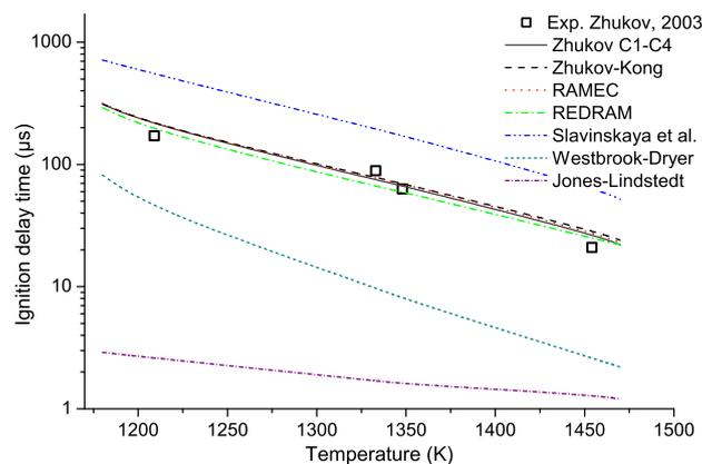
Figure 6: Comparison of different methane mechanisms with experimental data:<sup>42</sup> methane-air,  $\phi = 0.5$ , 150 atm.
