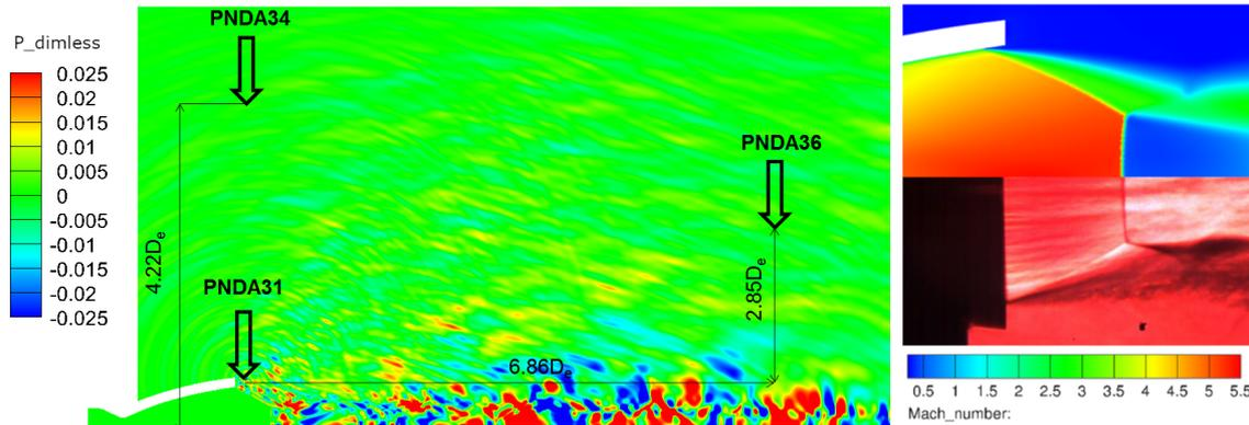
Figure 15: Right: Comparison of RANS simulation with Schlieren image. Left: Dimensionless pressure oscillations from CAA simulation and microphone positions relative to nozzle exit diameter.
