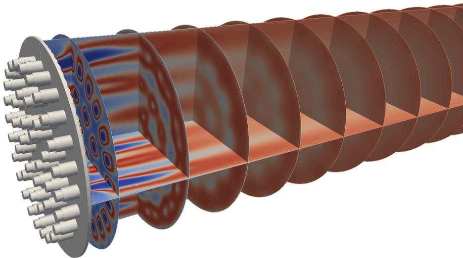
Figure 2: BKD combustion chamber simulation at a nominal combustion chamber pressure of 4.9 MPa
