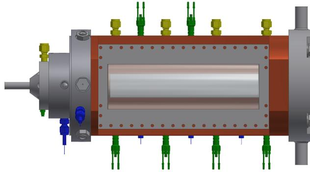
Figure 5: Preliminary design of a combustion chamber for numerical validation purposes
