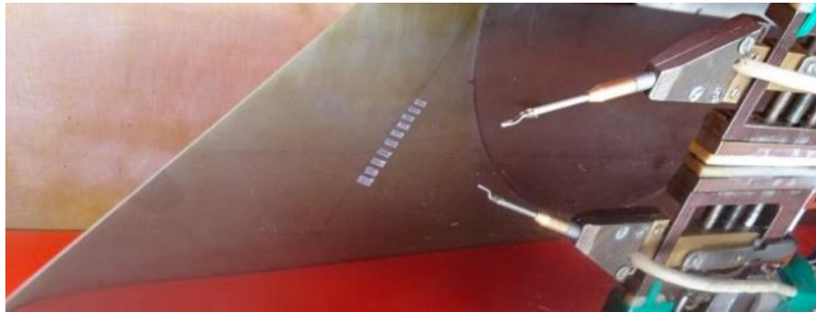
FIGURE 1. Photo of the swept wing model with roughness elements, hot-wire and traversing gear
