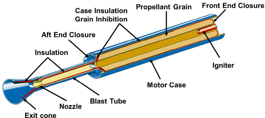
Figure 1: Typical elements of a solid rocket motor
