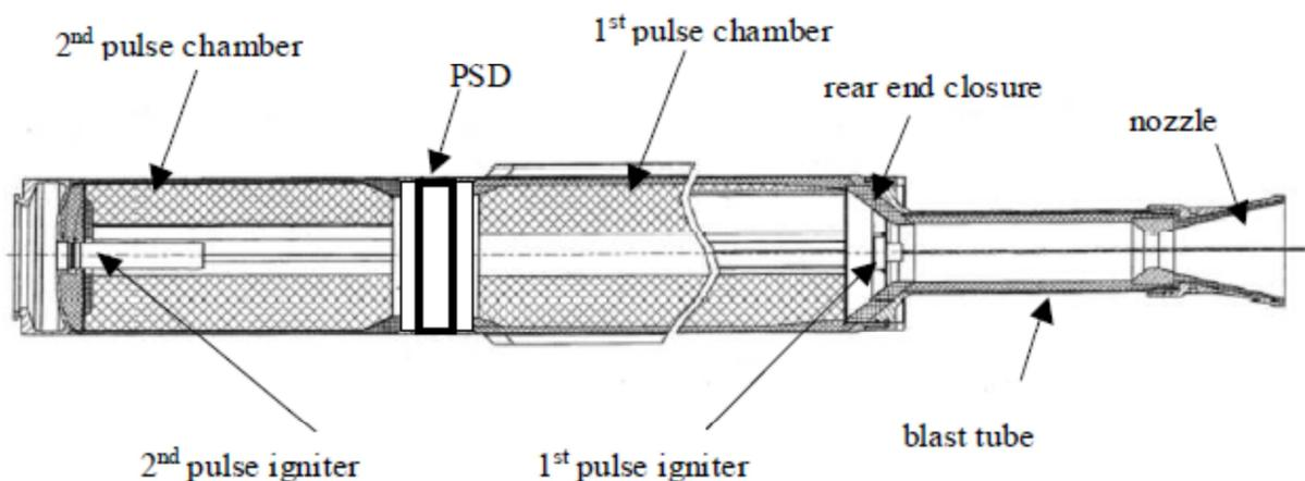
Fig. 6: Longitudinal cut of the flight demonstrator DPM SRM
