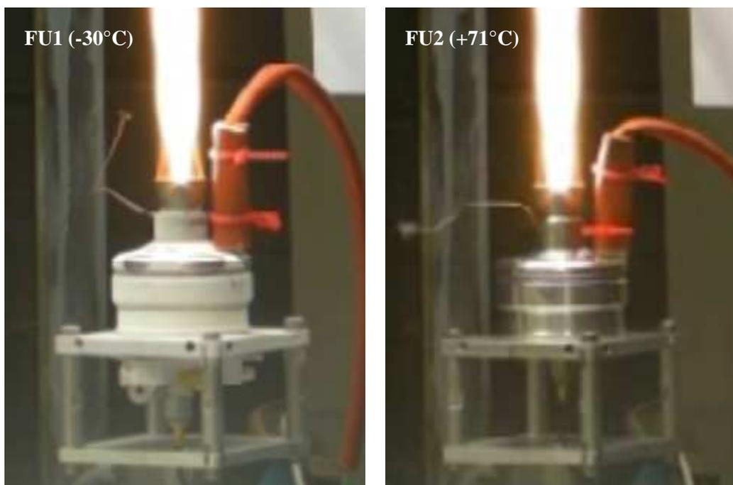
Fig. 4: Separation of the exhaust jet in the nozzle (Functional Tests FU1 and FU2)
