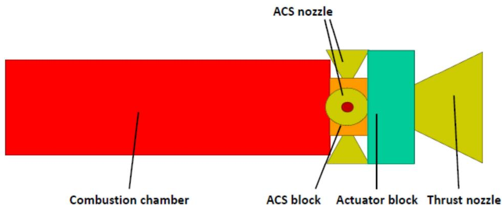
Fig. 5: Architecture of an SRM with TACS
