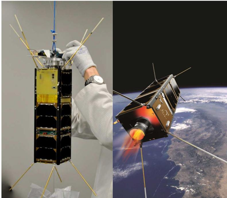
Figure 2: Picture of the D-SAT satellite and artist's impression of the de-orbiting manoeuvre
