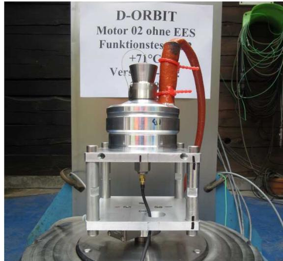
Fig. 3: Vertical test stand for all D-SAT the motor firings
