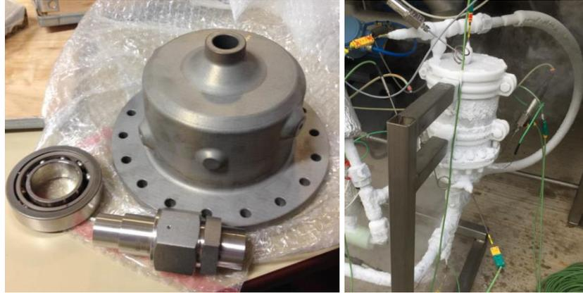
Figure 3: Lower assembly after the ALM-manufacturing process (left) and assembled demonstrator (right) undergoing a standard full-flush chill-down test sequence (right)
