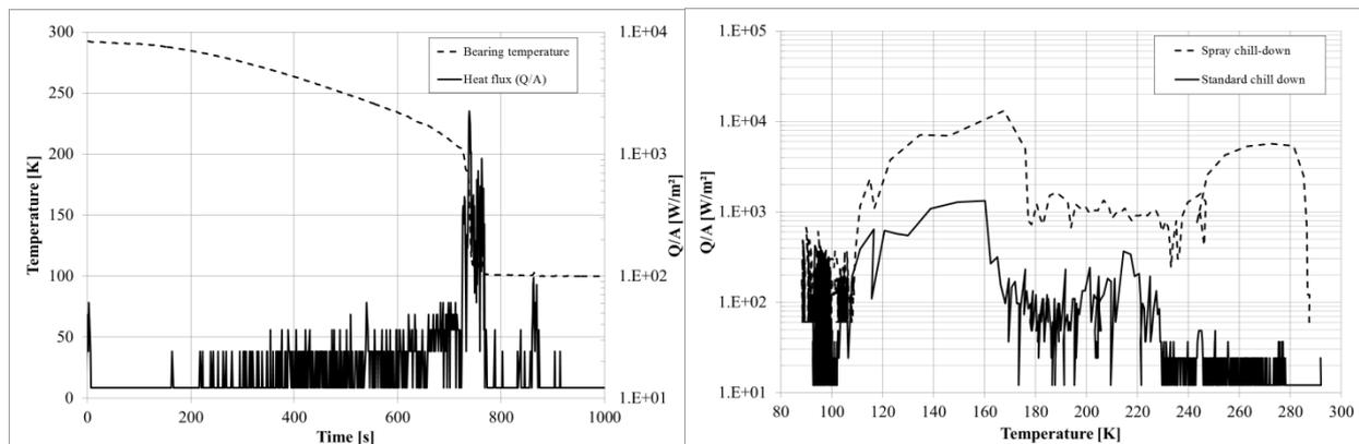
Figure 6: Ball bearing temperature and heat flux temporal evolution (left) and comparison of the boiling curves as a function of the chill-down methodology (right).
