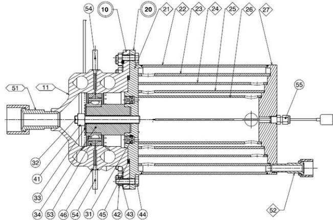
Figure 2: Cutaway of the spray chill-down demonstrator (labels are included in the text)
