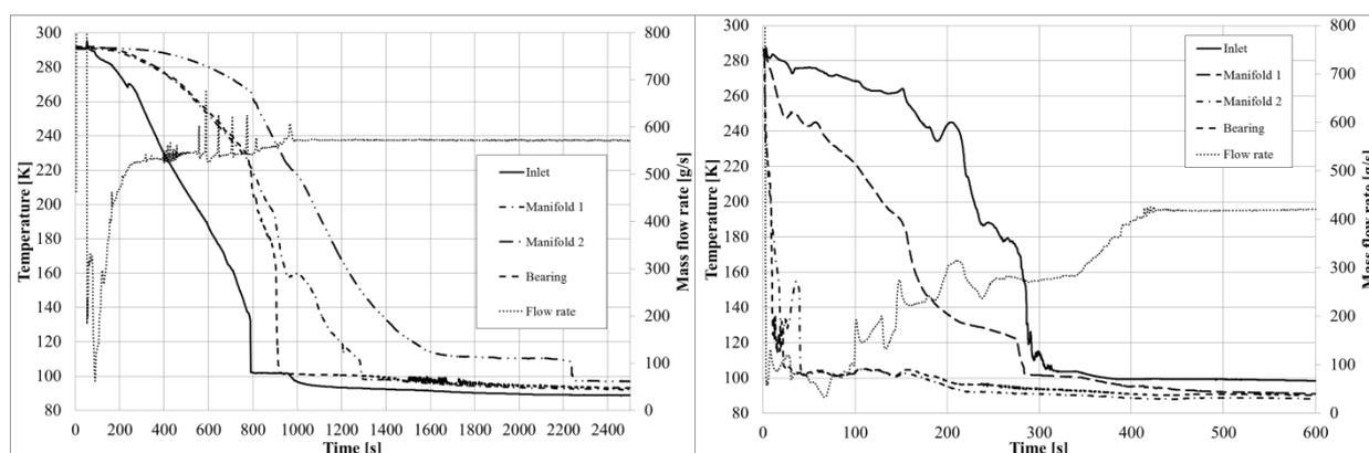
Figure 5: Temperature and mass flow rate temporal evolution during the standard full-flush chill-down (left) and during the spray chill-down (right).
