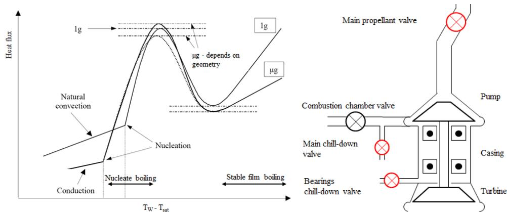
Figure 1: Boiling curve under 1-g and  $\mu$ -g conditions presenting the heat flux as a function of the wall to saturation temperature difference (left) and cryogenic turbopump classic chill-down architecture (right)
