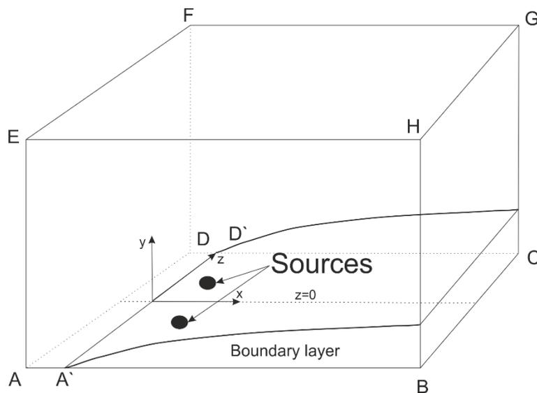
**Figure. 1** Scheme of flat plate model, coordinate systems used, sources and computational domain
