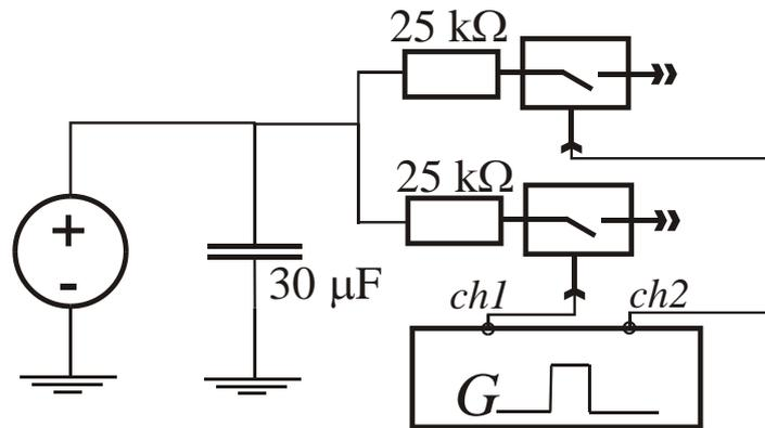
Figure. 2 The ignition circuit
