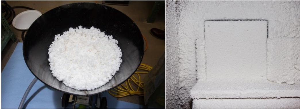
**Figure 6:** Aerogel-binder mix in the pump material container (left) and one of the as-sprayed plates (right).
