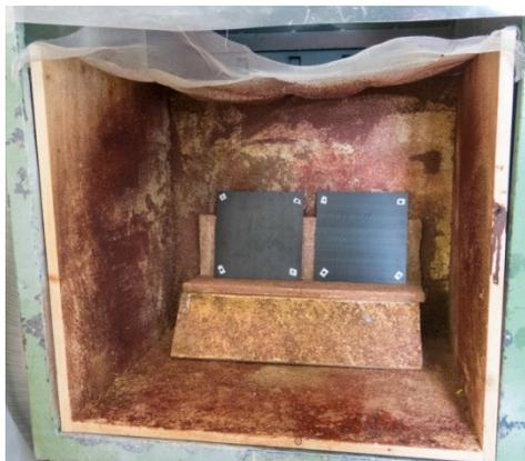
**Figure 2:** Ventilated spraying cabin with substrate plates ready to be coated.
