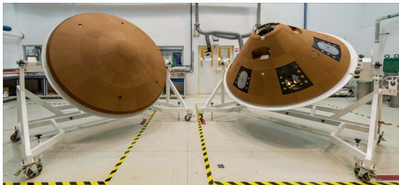
**Figure 1:** ExoMars Schiaparelli spacecraft with cork TPS. credit: ESA
