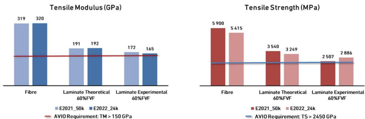
Figure 11: Tensile tests results in fibre direction for laminates produced with European IM carbon fibres
