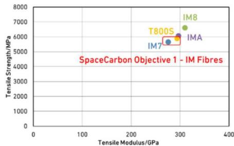
Figure 3: Commercial fibres versus SpaceCarbon objectives for launcher demonstrators
