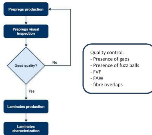
Figure 6: Flowchart for pre-prepregs and laminate production
