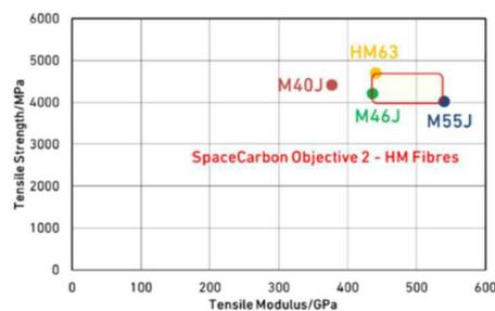
Figure 4: Commercial fibres versus SpaceCarbon objectives for satellite demonstrators
