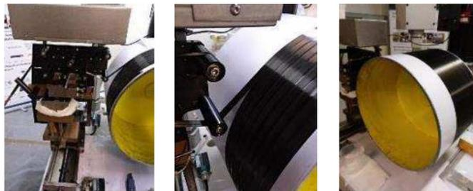
Figure 7: Lab scale prepregs manufacturing
