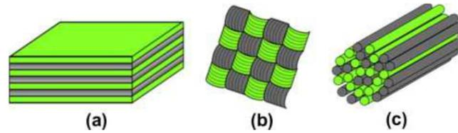
Figure 5: The three hybrid configurations: (a) interlayer, (b) intralayer, and (c) intrayarn
