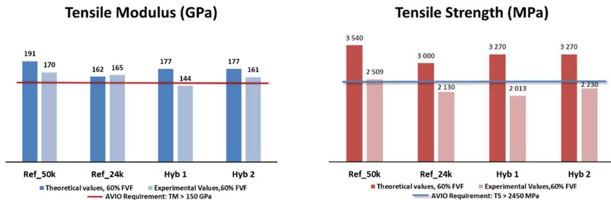
Figure 12: Tensile tests results in fibre direction for hybrid laminates produced with European IM carbon fibres and commercial fibres
