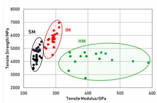
Figure 1: CF distribution according to their tensile strength and modulus
