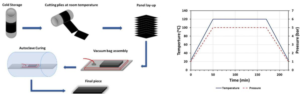
Figure 8: General prepreg processing flow (left) and conditions used in prepreg consolidation (right)
