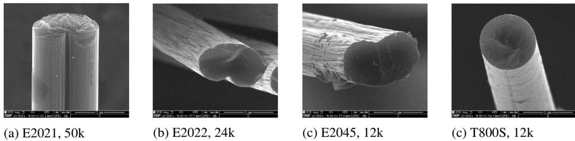
Figure 10: Cross-sectional geometry structure observations of carbon fibres for launcher applications
