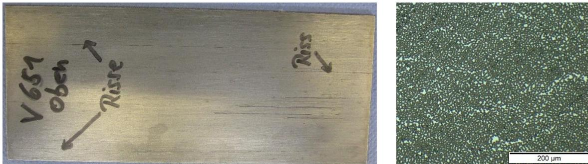
Figure 6. Resulting Al-MMC coupon plate after manufacturing (left) and cross-section of the Al-infiltration.
