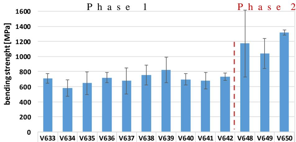
Figure 9. Bending test results of coupon plate test samples V633 – V650
