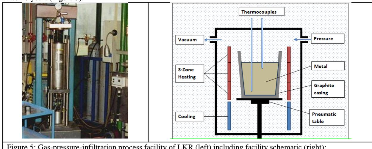
Figure 5: Gas-pressure-infiltration process facility of LKR (left) including facility schematic (right);
