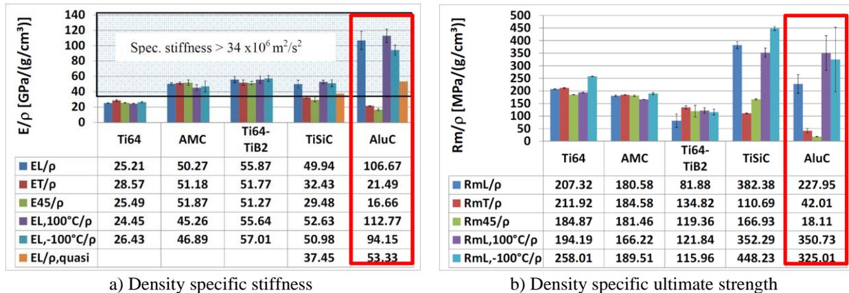
Figure 1: Comparison of (a) density specific stiffness and (b) density specific strength of the assessed high-performance materials; LKR material AluC in red Box; [1]
