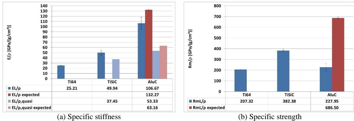
Figure 3: Measured (a) specific stiffness and (b) strength of Ti64, TiSiC and LKR Al-MMC (blue) compared to theoretical max. values (red) in uni-directional (L) and quasi-isotropic layup (transparent).
