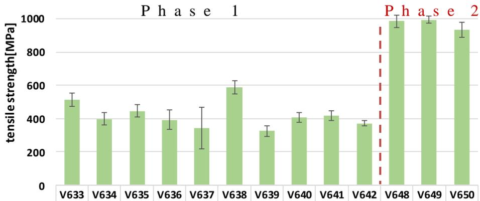
Figure 11. Tensile test results of coupon plate test samples V633 – V650
