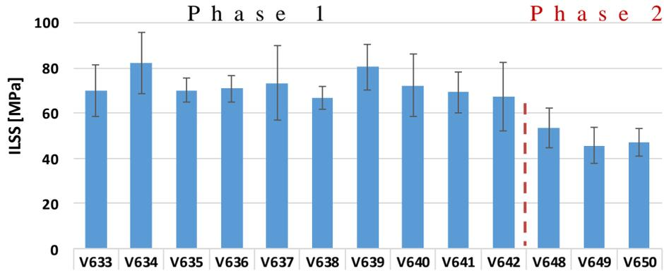
Figure 8. Interlaminar shear test results of coupon plate test samples V633 – V650
