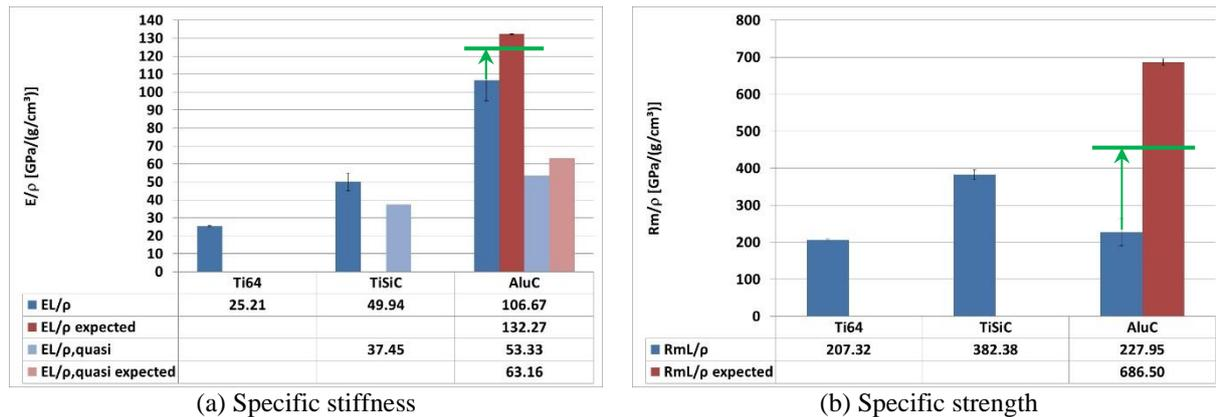
Figure 12: Improved (a) density specific stiffness and (b) density specific ultimate strength (green horizontal line) achieved compared to Ti64, TiSiC and AluC values (blue) and theoretical values (red) of (see also Figure 3).
