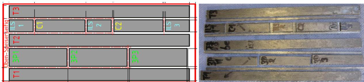
Figure 7. Sample plan (left) and final, milled Al-MMC samples out of coupon plate for mechanical testing.
