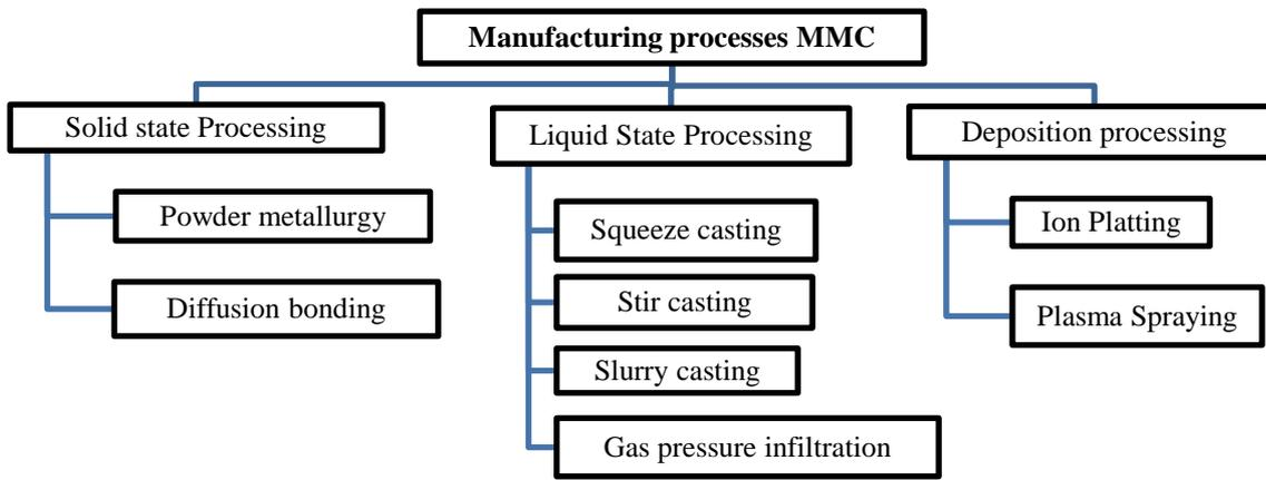
Figure 4. Most common MMC manufacturing processes
