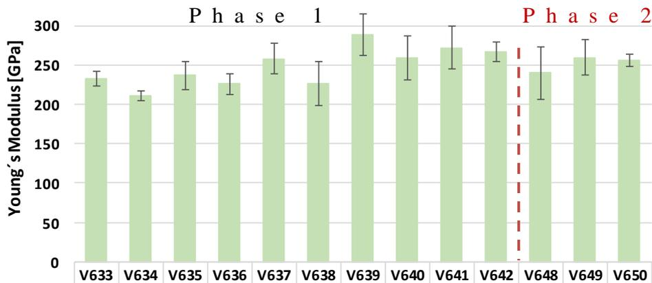
Figure 10. Young's Modulus results of coupon plate test samples V633 – V650
