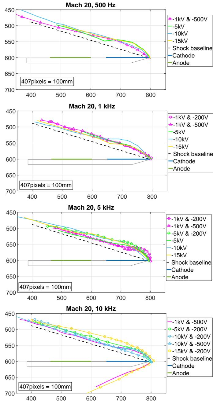
Figure 8: Shock wave shapes determined for different applied output pulse voltages: 500 Hz, 1 kHz, 5 kHz and 10 kHz.
