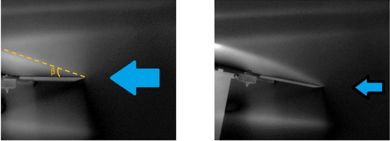
Figure 3: iCCD image of the flat plate in the Mach 20 flow with an angle of attack of  $0^\circ$ , *i.e.* the baseline (left) and with an angle of attack of  $-10^\circ$ . (right)
