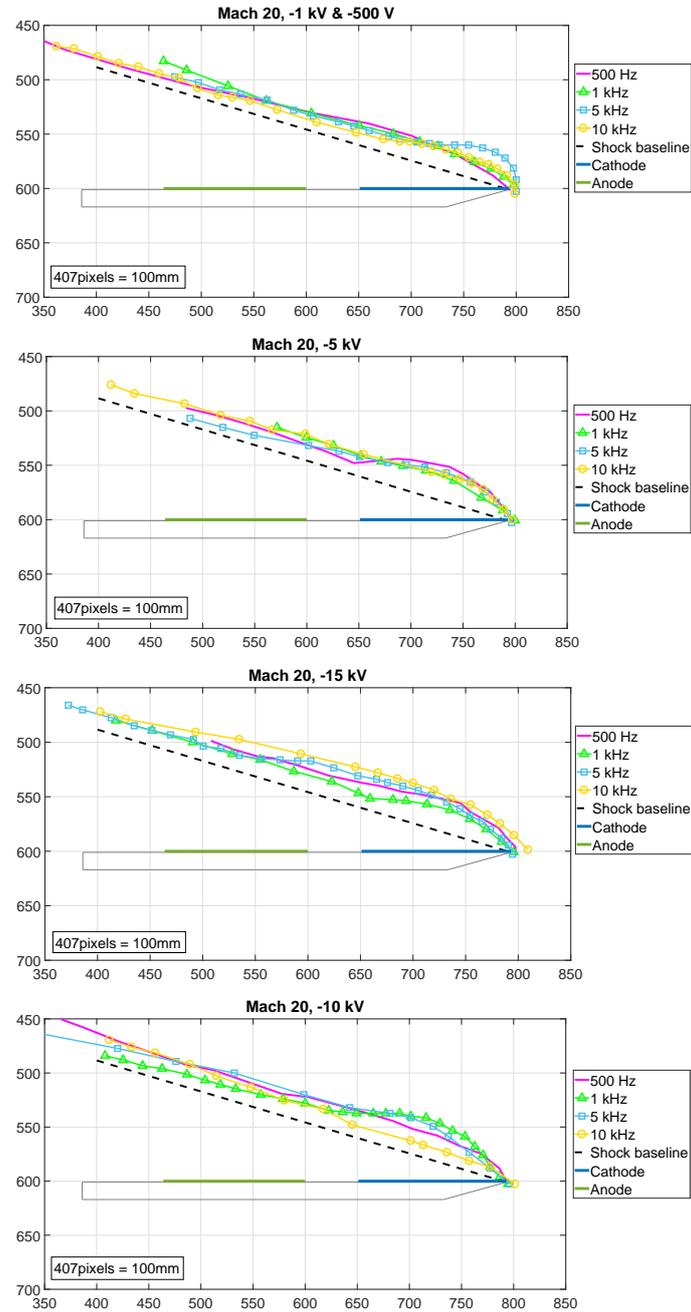
Figure 9: Shock wave shapes for different repetition rate pulse:  $-1\text{ kV}$ ,  $-5\text{ kV}$ ,  $-10\text{ kV}$  and  $-15\text{ kV}$ .
