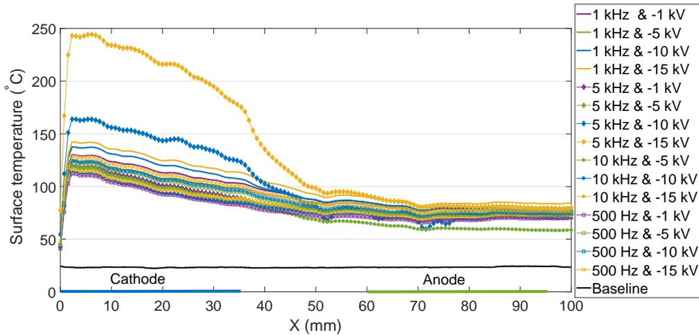
Figure 7: Surface temperatures on the upper surface of the flat plate for the different cases studied.
