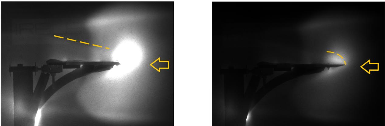
Figure 6: iCCD images of the flowfield modified with a discharge of  $-1$  kV and 5 kHz, recorded with two different settings: (left) camera gain of 150 and camera gain of 110(right). The yellow dashed line represents the shock wave.
