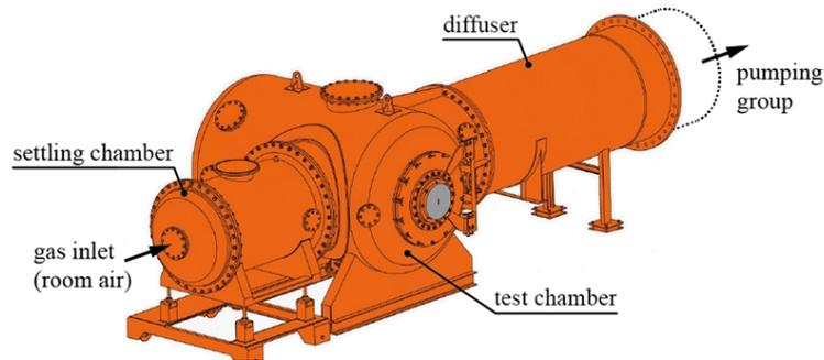
Figure 1: The Marhy wind tunnel lay-out.
