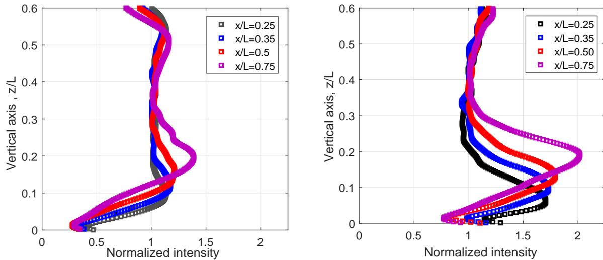
Figure 4: Experimental density profiles retrieved from the iCCD images for an angle of attack of  $0^\circ$  (left) and an angle of attack of  $-10^\circ$  (right).
