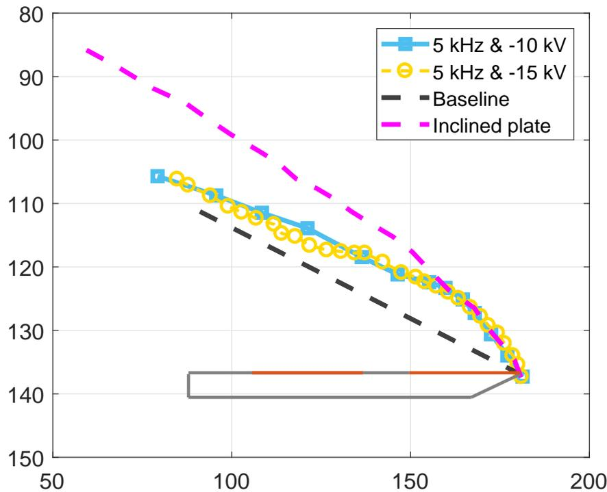
Figure 10: Comparison of the shock wave shapes obtained with pulsed plasma actuator (5 kHz and  $-10$  and  $-15$  kV) and with the flat plate at  $-10^\circ$  angle of attack.
