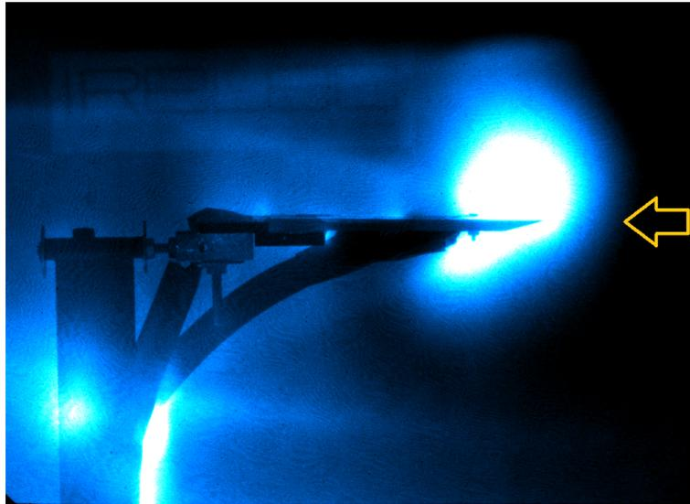
Figure 5: iCCD image of the pulsed discharge for 10 kHz and  $-1$  kV in the hypersonic flow.
