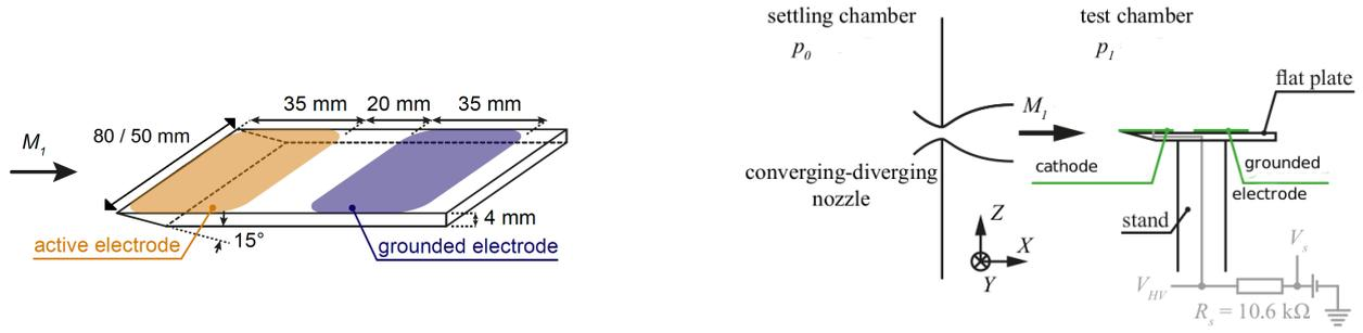
Figure 2: Scheme of the flat plate with the plasma actuator (left) and Experimental set-up (right).
