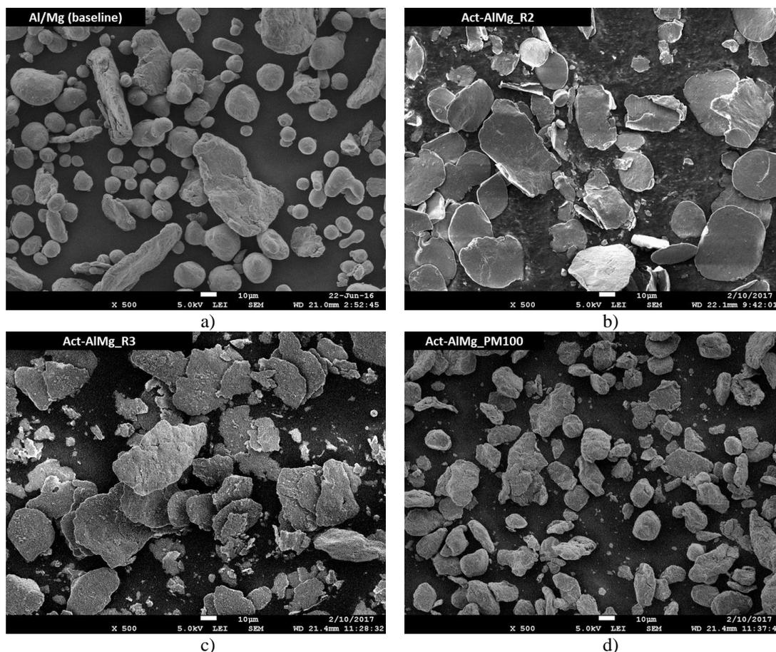
Figure 2. SEM images of activated powders. The virgin mixture and a powder activated through a standard technique (Act-AlMg\_PM100) are reported for comparison.
