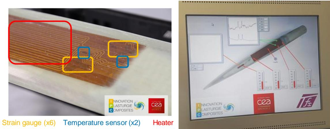
Figure 10: component's description and interface display
