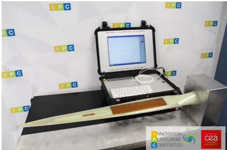
Figure 9: overview of blade part and acquisition/control system
