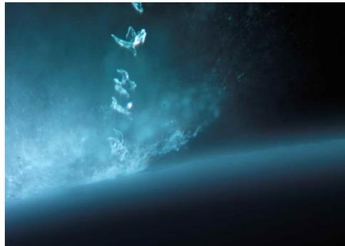
Figure 13: Droplets of 1 mm splashing on the moving airfoil DBK002 at 90 m/s.
