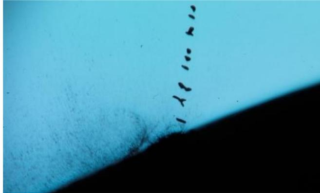
Figure 15: Example of the image taken by shadowgraph technique with the micro-flash and model velocity 80 m/s.
