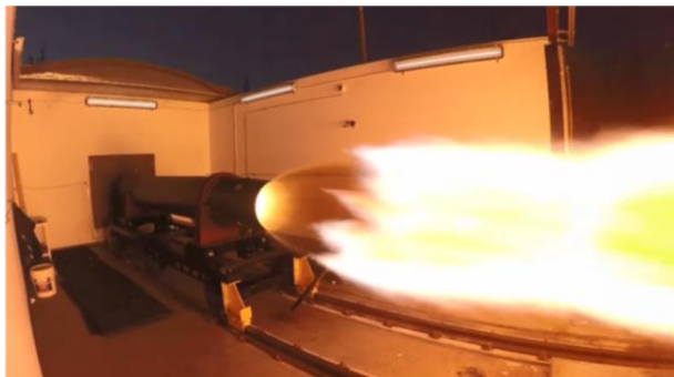
Figure 3 Test fire of 500kN motor in 2018
