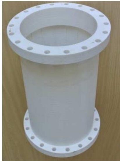
Figure 8: 3D-printed polymer specimen
