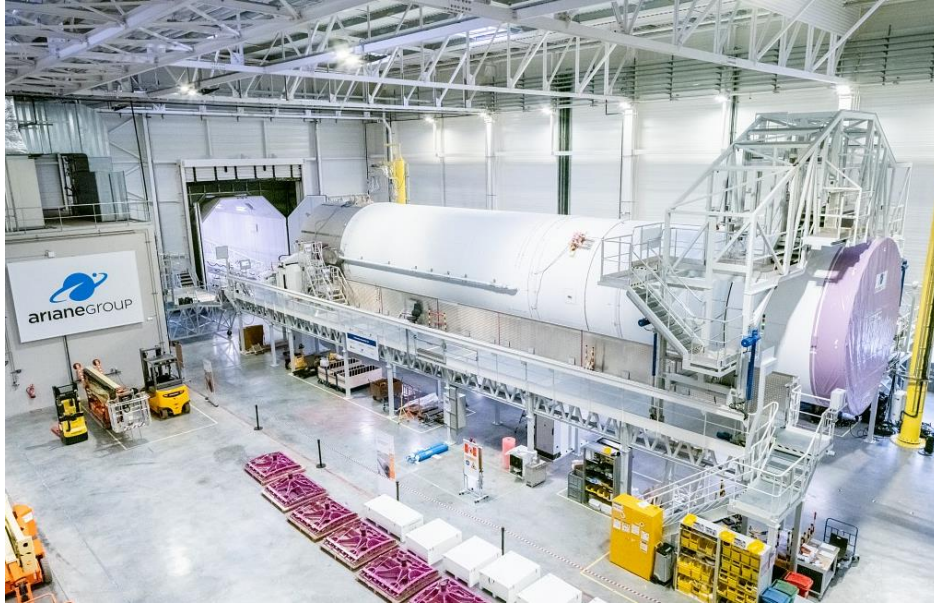
Figure 4: Ariane 6 lower-stage cryogenic tanks
