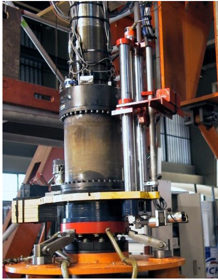
Figure 10: testing machine for compression with pressure
