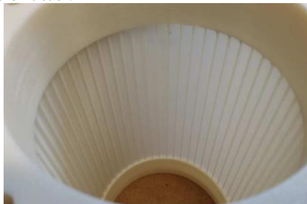
Figure 20: 3D-printed polymer stiffened shell
