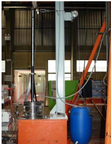
Figure 11: testing machine for shear/bending test with pressure
