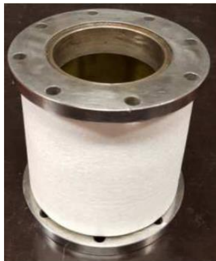
Figure 9: Specimen with a foam coating
