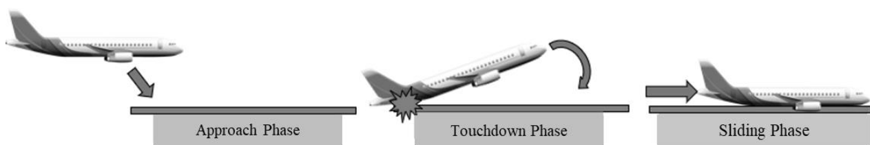
Figure 1: Phases of an aircraft emergency landing (gear retracted)
