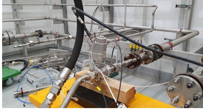
Figure 8: Flow and maneuvering test setup
