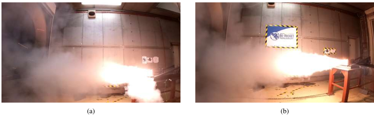
Figure 5: GoPro view of the static firing test: (a) PRO38 and (b) PRO75.
