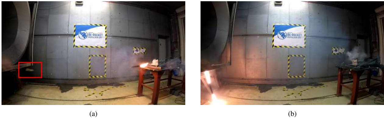
Figure 8: GoPro footage of the failed static Test 5 for the PRO38 motor. The failure was caused by the nozzle being ejected at ignition. (a) Frame showing the nozzle ejection immediately after the pressure rise, and (b) the propellant grain burning outside the motor casing.
