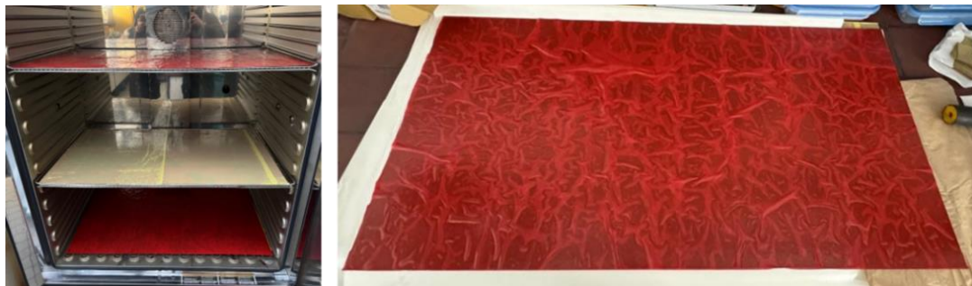
Figure 2: Lamination of SS sheets with adhesive film in an oven
