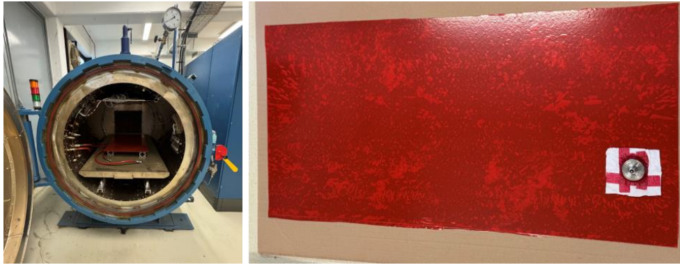
Figure 3: Lamination of SS sheets with adhesive film in an autoclave
