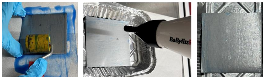
Figure 8: Coating and drying of photoresist layer on EB-perforated specimen
