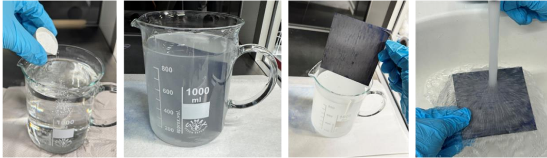
Figure 10: Development of photoresist; preparation of solution, dipping of coated part in solution and washing
