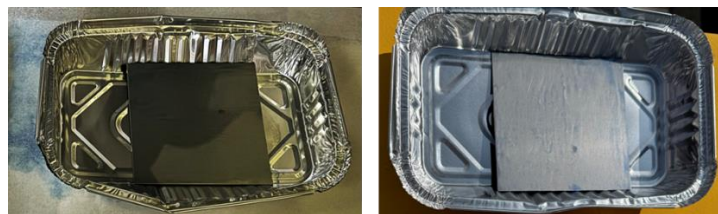
Figure 9: Specimen kept in darkness for drying (left) and in sunlight for curing (right)
