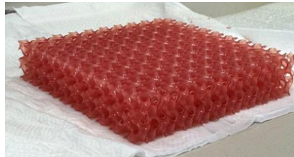
Figure 11: 3D printed gyroid structure for HLFC suction panel
