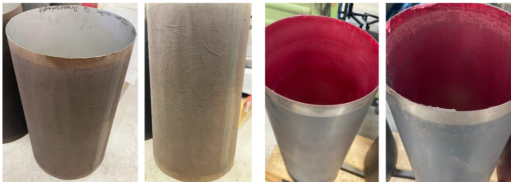
Figure 4: EB perforated SS sheet with adhesive on outer side (left) and adhesive on the inner side (right)
