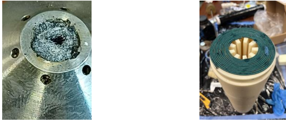
Figure 13 Slug deposited at the igniter nozzle (left), visco fuse glued on top of the grain (right)
