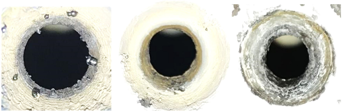
Figure 16 Nozzle throat diameters after firing, showing a stepwise erosion of the HT-2D nozzle surface, corresponding to the fabric lay-up, but a homogeneous increase of the diameter (left, T6). Less erosion but inhomogeneous increase of the UHM – SF throat diameter (T5) after 380 s (middle) and 644 s (right) firing time.
