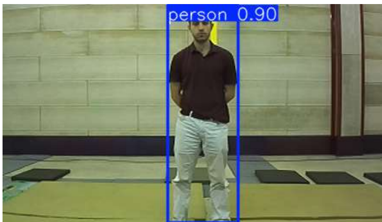
Figure 1: YOLO's result on the RGB images. The number indicates the level of confidence in the detection.
