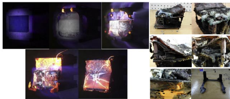
Fig. 4: Typical results from tests in arc-jet facilities [17]
