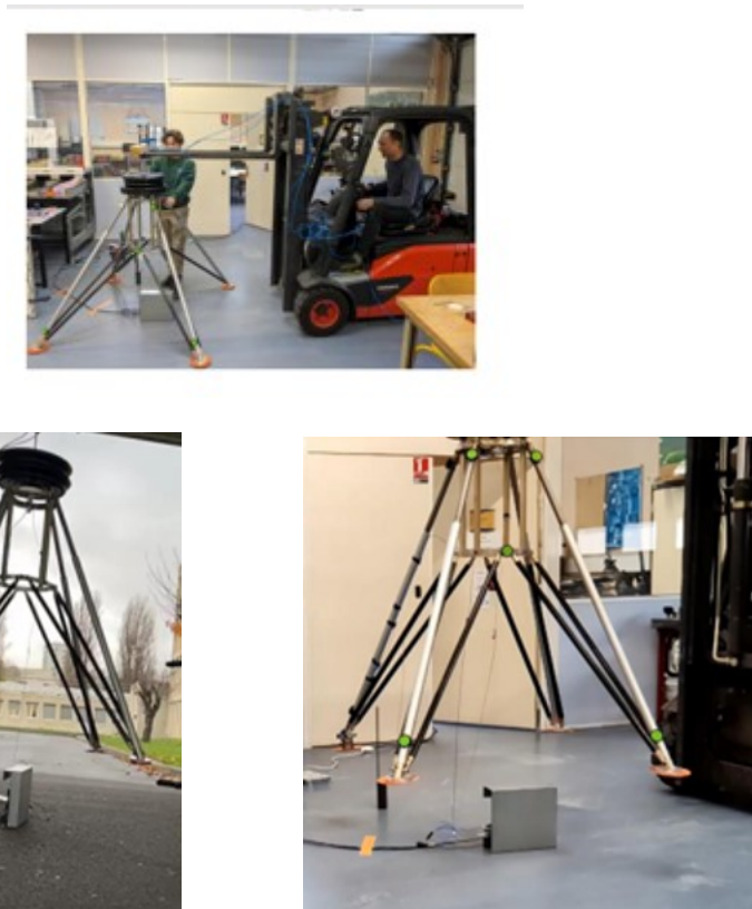
Figure 12: Landing legs tests: damping system identification
