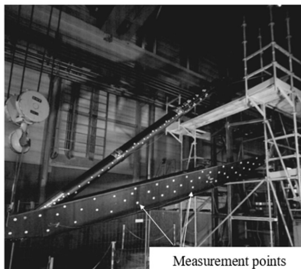
Figure 5: Complete Landing Leg with optical measurement points
