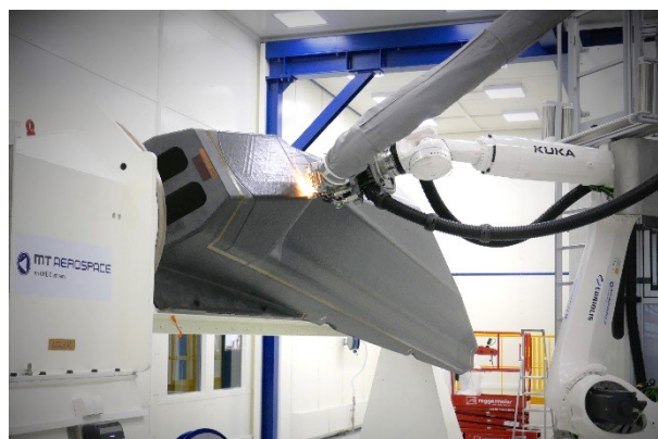
Figure 4: AFP layup of LLAY on AM tooling
