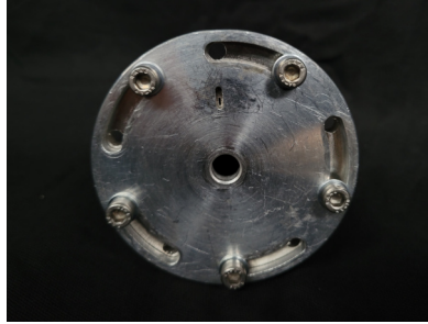
Figure 11: depowdering flange with slot for single cooling channel
