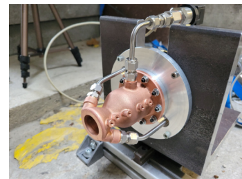
Figure 20: copper engine mounted on the test bench
