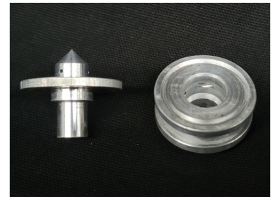
Figure 3: Coaxial swirl injector assembly. Left: Inner swirl chamber; Right: Outer swirl chamber
