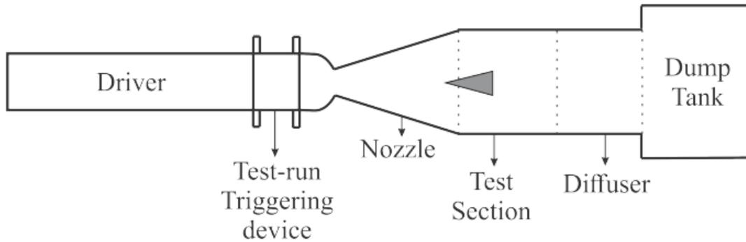
Figure 7: Ludwig tube simplified layout [17].
