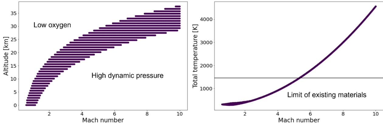
Figure 5: Flight corridor analysis for an airbreathing vehicle.
