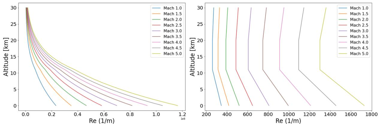
Figure 6: Dimensional analysis for the proposed flight corridor.
