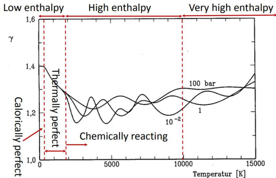
Figure 4: Variation of the isentropic exponent,  $\gamma$ , of air with temperature and pressure [12].
