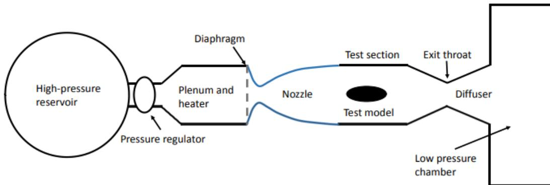
Figure 9: Blown down wind tunnel basic layout [12].
