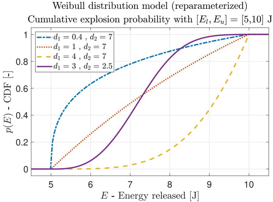
Figure 4: Example of Weibull distribution estimation on the cumulative ignition probability  $p(e)$  after reparametrization. Legend order: concave, quasi-linear, convex, S-type
