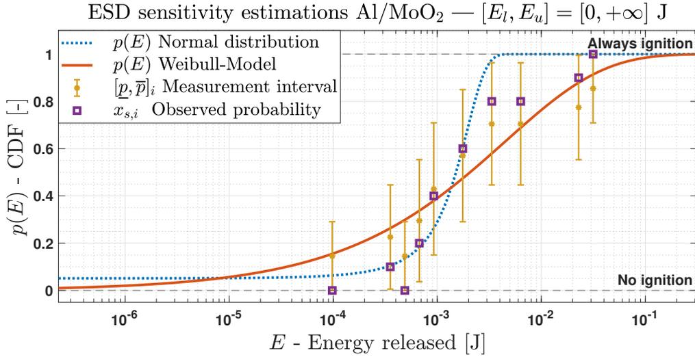
Figure 5: Comparison of the ignition sensitivity estimation models
