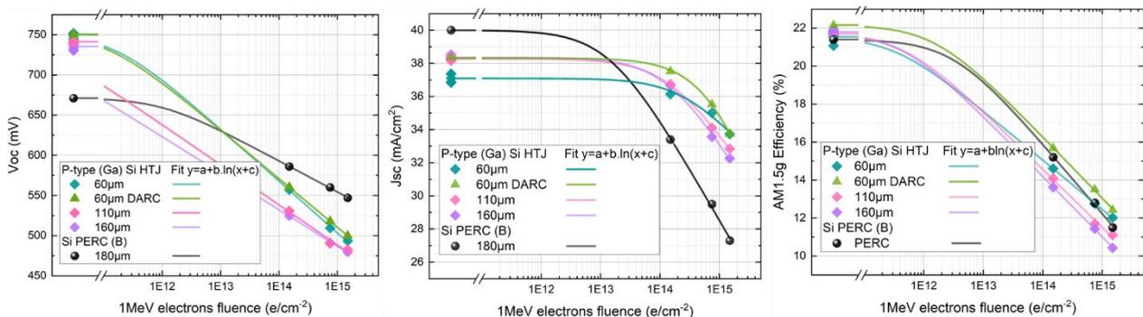
Figure 3 - Variations of  $V_{oc}$ ,  $J_{sc}$  & Efficiency as measured in-house under AM1.5G spectrum at room temperature for p-type Ga-doped Si heterojunction solar cells with various thicknesses. Comparison with commercial PERC cell.
