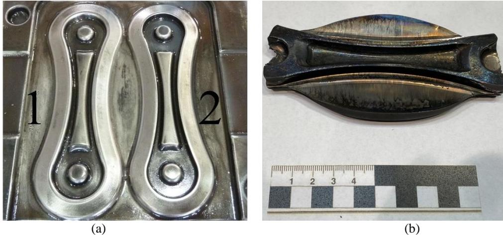
Figure 3: Showing the used forging die, including the sequence of forging steps (a) and a forged part made from Mg-20Li-15Al-1Ca-0.5Y alloy (b).
