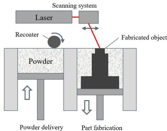
Figure 1: Schematic representation of the laser-powder bed fusion (L-PBF) process, based on [8]
