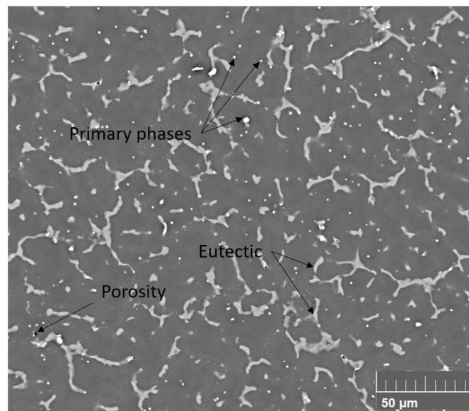
Figure 6: Typical microstructure of a Mg-Al alloy in as-fabricated state produced via waDED
