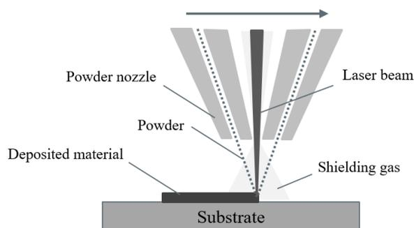
Figure 3: Schematic representation of the pDED process, based on [18]
