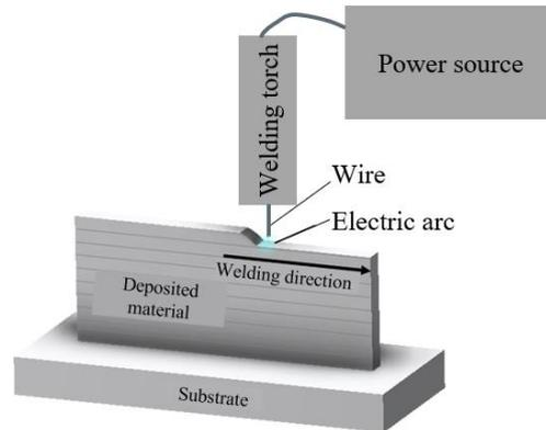
Figure 4: Schematic representation of the wire-arc directed energy deposition process, based on [20]
