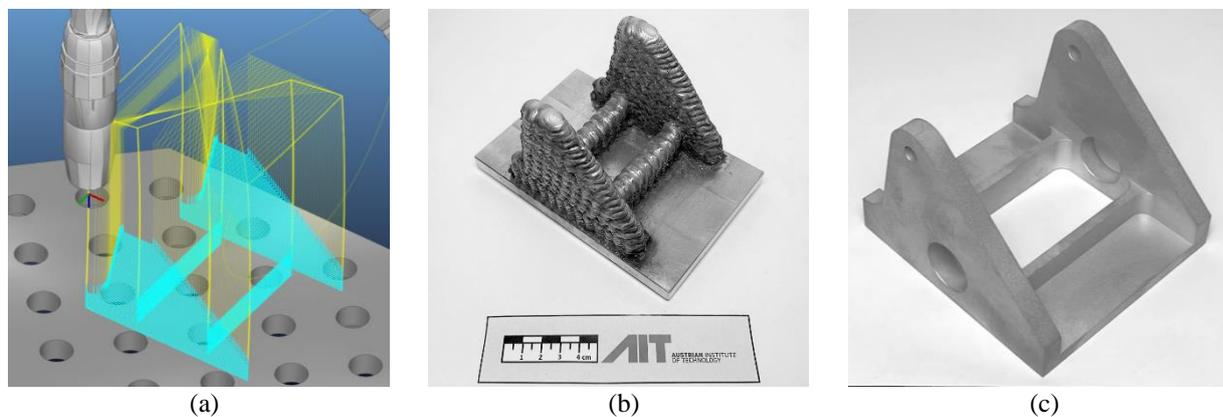
Figure 7: Single steps for the production of a waDED part: (a) Robot motion programming, (b) body-in-white, (c) final part after machining
