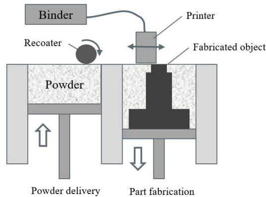
Figure 2: Schematic representation of the binder jetting process, based on [16]
