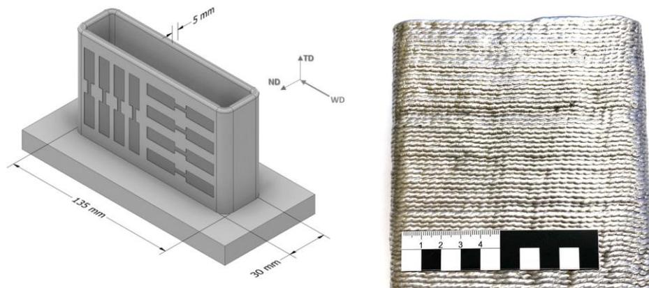
Figure 5: Schematic representation of thin-walled structure produced via waDED incl. sample extraction position (left) [21]. Front view of manufactured sample (right).
