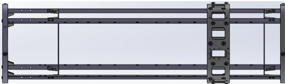
Figure 13: SERA4 avionic section skeleton
