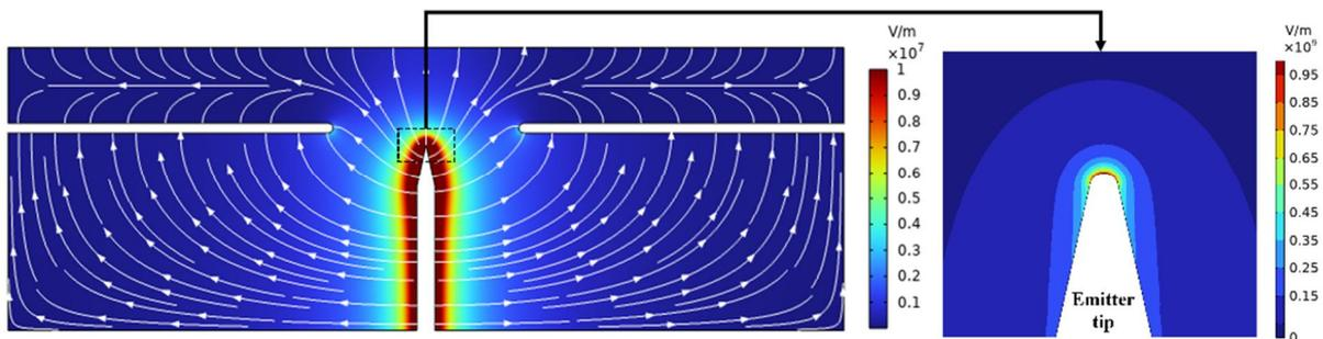
Figure 4: Electric field distribution for a single needle emitter
