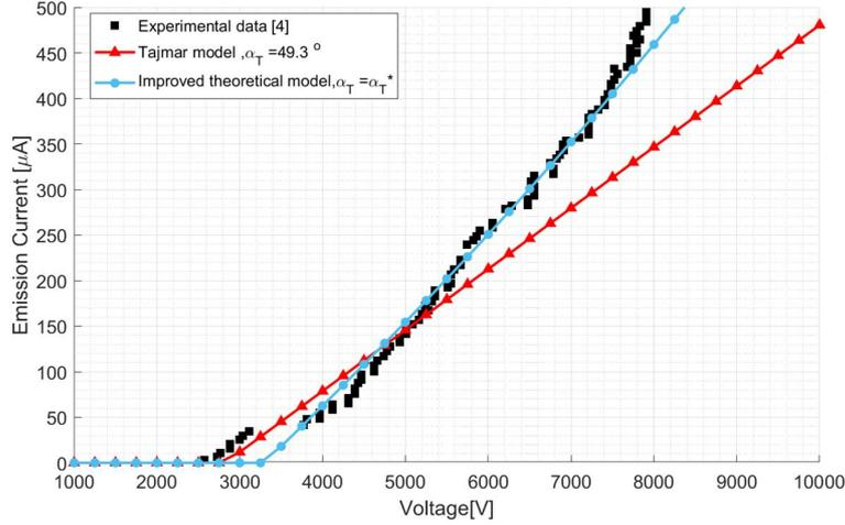
Figure 2: Comparisons of emission current-applied voltage characteristics for a single needle emitter
