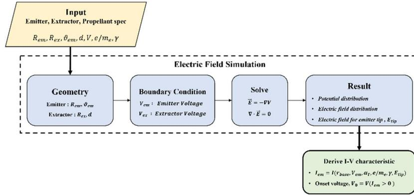
Figure 3: Flowchart of electric field simulation
