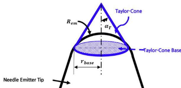
Figure 1: Taylor cone on needle emitter tip
