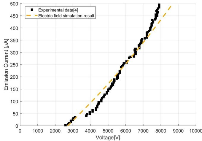
Figure 5: Comparison of emission current-applied voltage characteristics between simulation and experiment[4]
