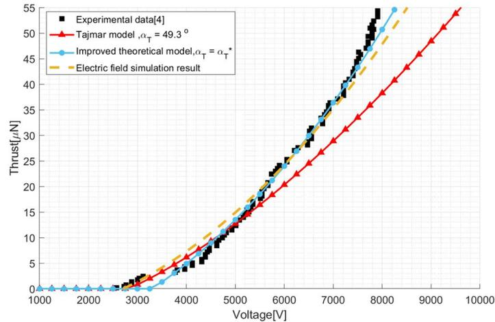
Figure 6: Comparisons of thrust-applied voltage characteristics for a single needle emitter
