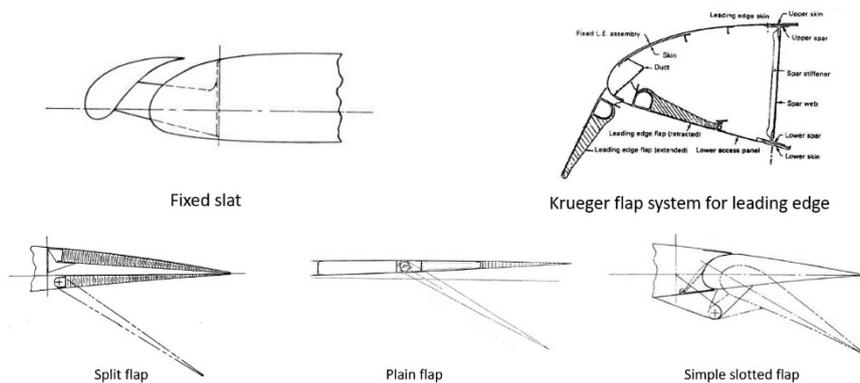
Figure 2: Conventional high lift devices for leading and trailing edges
