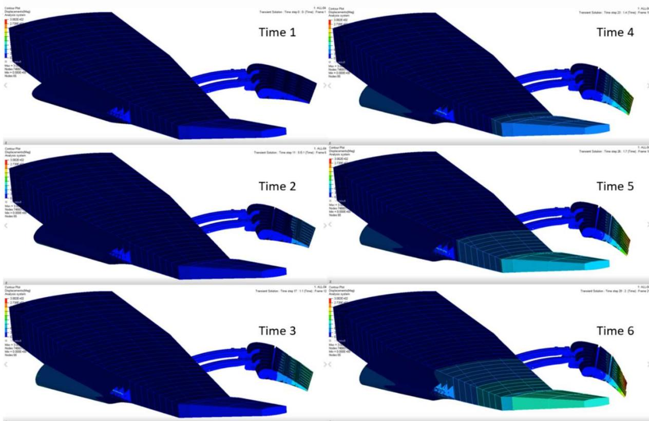
Figure 16: Motion and deformation of the full wing including the wingtip
