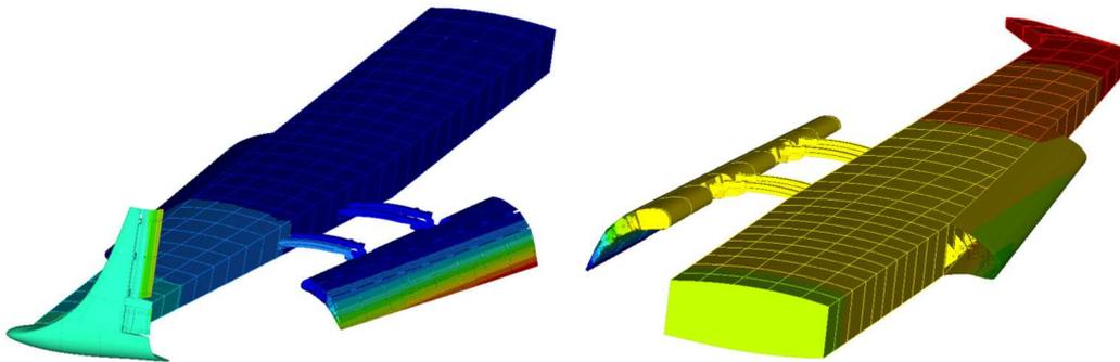
Figure 12: General views of the deployed mechanisms for the morphing wing model
