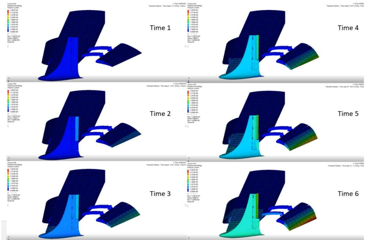
Figure 14: Motion and deformation of the full wing including the winglet
