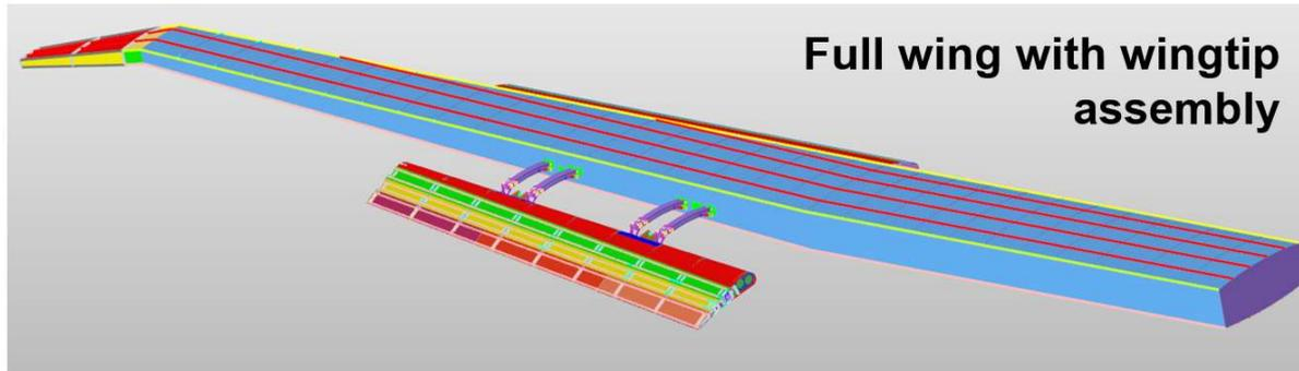
Figure 15: Wingtip mounted on the wing
