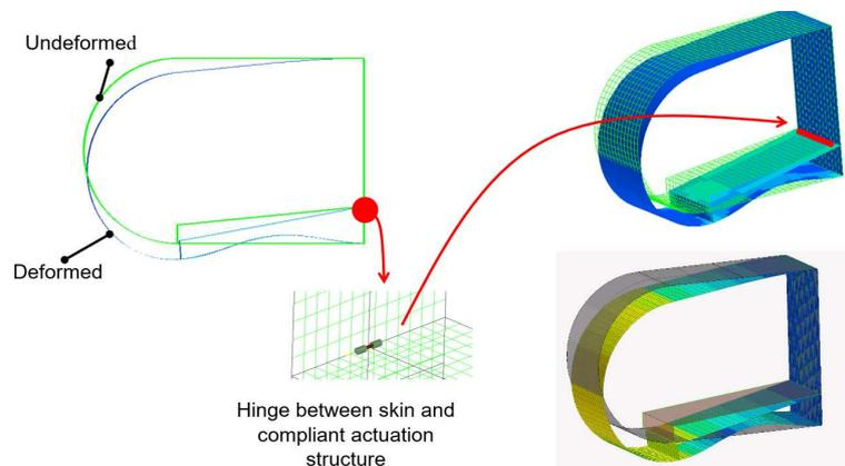
Figure 7: Using SAMCEF to develop a first (simple) model of a droop nose
